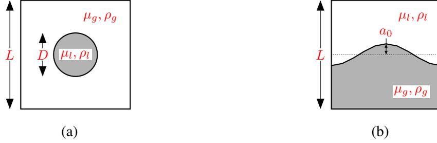
Figure 4.8: (a) Computational setup for spurious current test case in Sec:4.3.1. (b) damping capillary wave in Sec4.3.2
