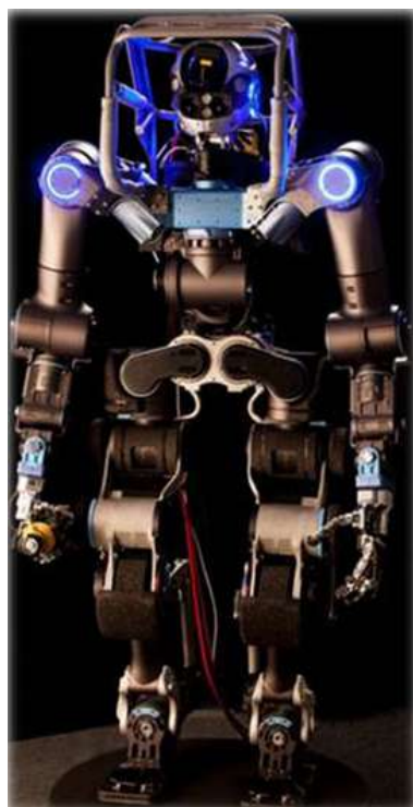
FIGURE 2.13 – Robot bipède WALKMAN.
