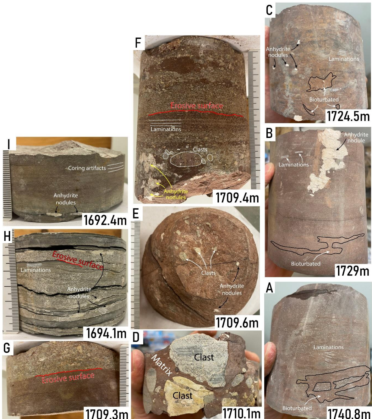
Figure 53: Representative selection of retrieved core samples from the “Éocène basal”. (A) Intensely bioturbated red clayey limestone with burrows and deformed laminations. (B, C) Similar to (A), but with anhydrite nodules. (D) Pebbly mudstone with sub-angular to sub-rounded Jurassic limestone clasts. (E) Pebbly mudstone with small and
