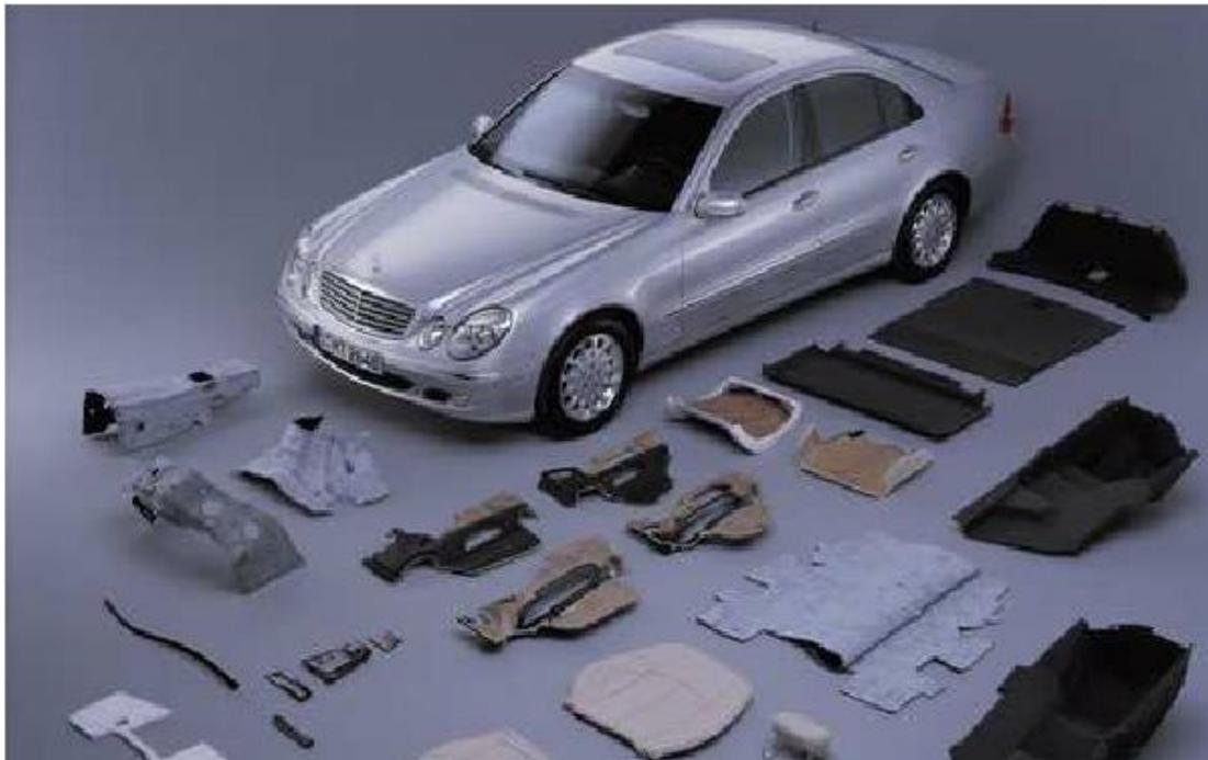
Figure 1.1 Automobile components made of natural fiber composites [12].
