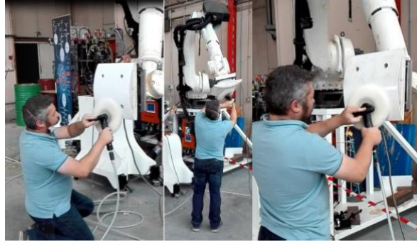
Figure 71. Polishing activity on a kistler sensor following various postures, recording of the forces.
