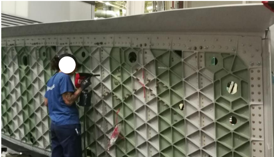
Figure 50. The task involves performing vertical assembling operations in arm-elevated posture.
