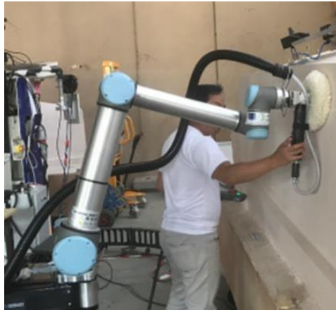
Figure 73. An operator is manipulating the polishing system to learn the window to polish
