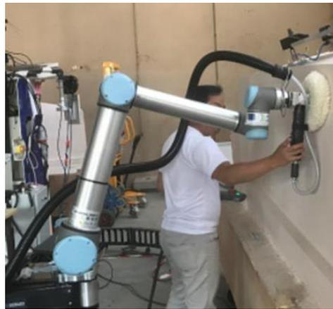
**Figure 73.** An operator is manipulating the polishing system to learn the window to polish
