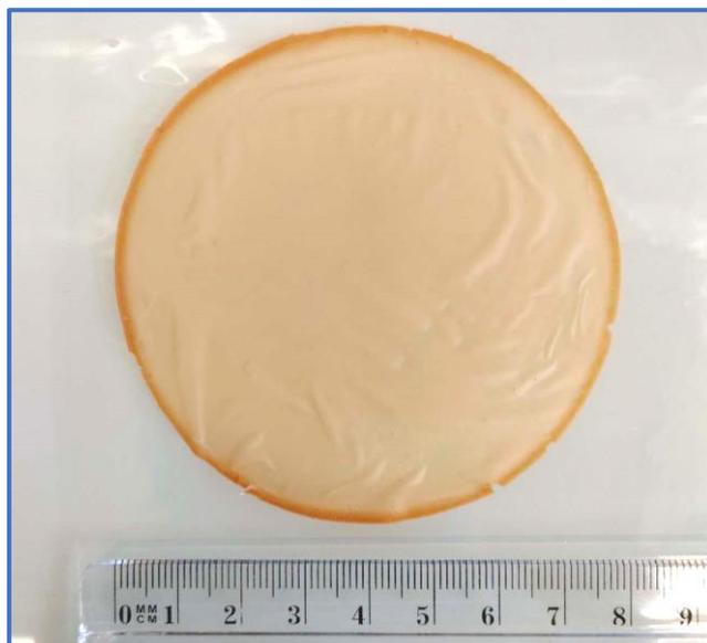
Figure 41. SIPE membrane with mPEGME-PTFSIVE and PVDF-HFP with a ratio of 70:30.
