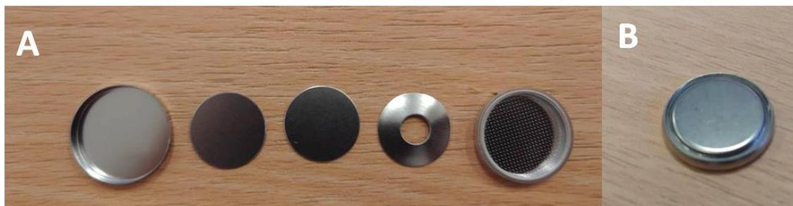
Figure 134. (A) Parts of CR2032 type coin cell. From left to right, the parts are bottom shell, spacer of 1mm , spacer of 0.5 mm, spring, top shell with sealing ring, respectively. (B) A CR2032 type coin cell after assembly.
