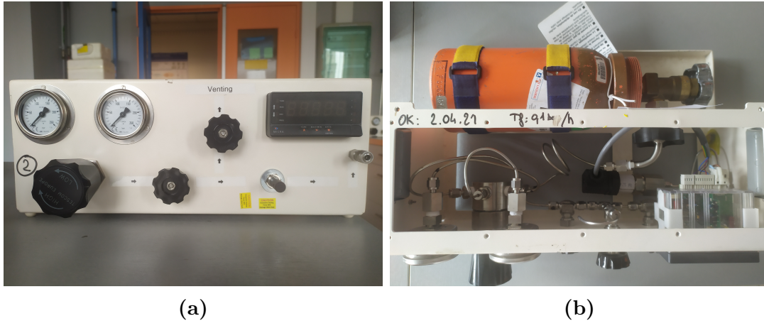
Figure 2.2: (a) Front and (b) top views of the gas supply device used for inflating the DAC membrane. The set-up is connected to a small gas bottle fill with helium with a maximum pressure of 150 bars.
