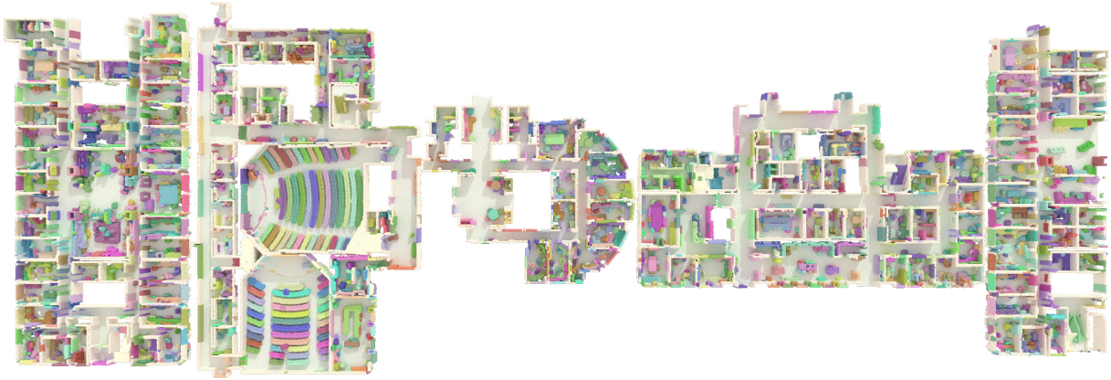
Figure 1.1 – Large-Scale 3D Scene Understanding. We develop methods for the efficient semantic analysis of large 3D point clouds. Other methods analyze indoor 3D scenes room by room, ours can consider hundred-room buildings at once, in a few seconds on a single GPU.
