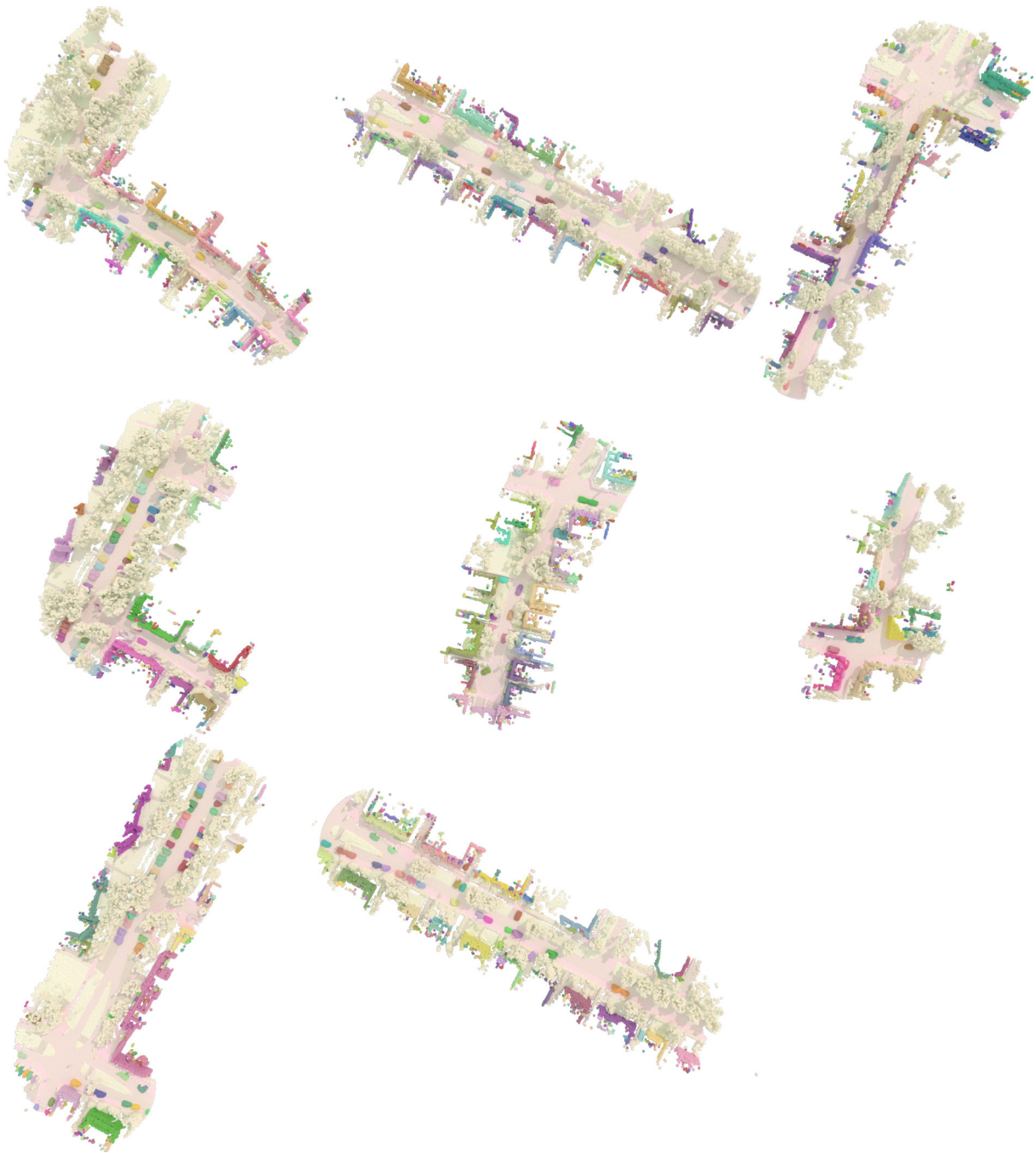
Figure 4.8 – Large-Scale Inference on KITTI-360. Largest scan that SuperCluster can segment in one inference on an A40 GPU: 7.5 tiles , 11.0m points , 414k superpoints , 602 target objects , and 1947 predicted objects . Inference takes 6.6 seconds .
