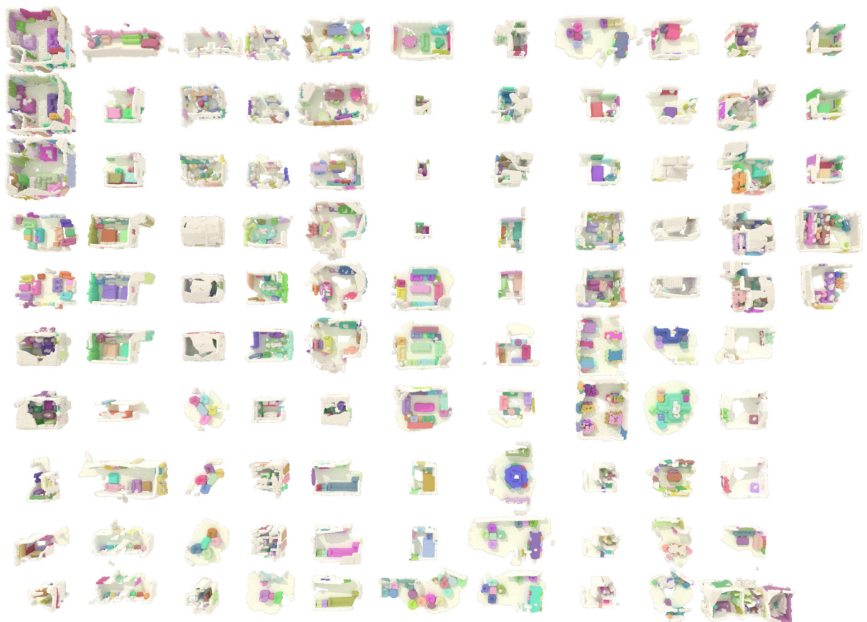
Figure 4.6 – Large-Scale Inference on ScanNet. Largest number of scans that SuperCluster can segment in one inference on an A40 GPU: 105 scans , 10.9m points, 398k superpoints , 1683 target objects, and 2148 predicted objects. The inference takes 6.8 seconds.
