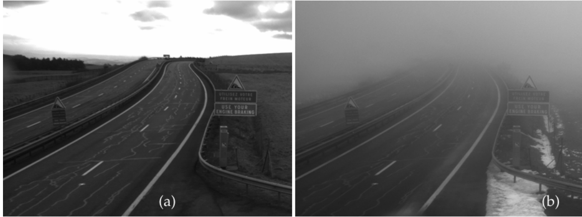
Figure 1.4: Real camera images taken from a section of the French A75 highway (at the Col de la Fageole point) without fog (a) and with fog (for visibility 156 m, (b)), both images are in grayscale (see [60]).
