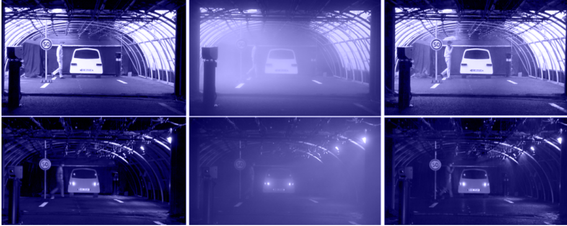
Figure 1.11: Some tests of sensor detection in both daylight and nighttime conditions in the presence of fog.
