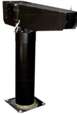
Figure 1.12: The transmissiometer DEGREANE HORIZON TR30 used in the PAVIN Fog&Rain Platform
