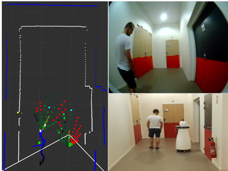
Figure 4.1: Snapshot from a lab-setting experiment from our person-following work (Scales et al., 2020). Left: visualisation of the joint person-robot planning. The position resulting from applying the optimal control is marked in light blue. Right: onboard and external views.
