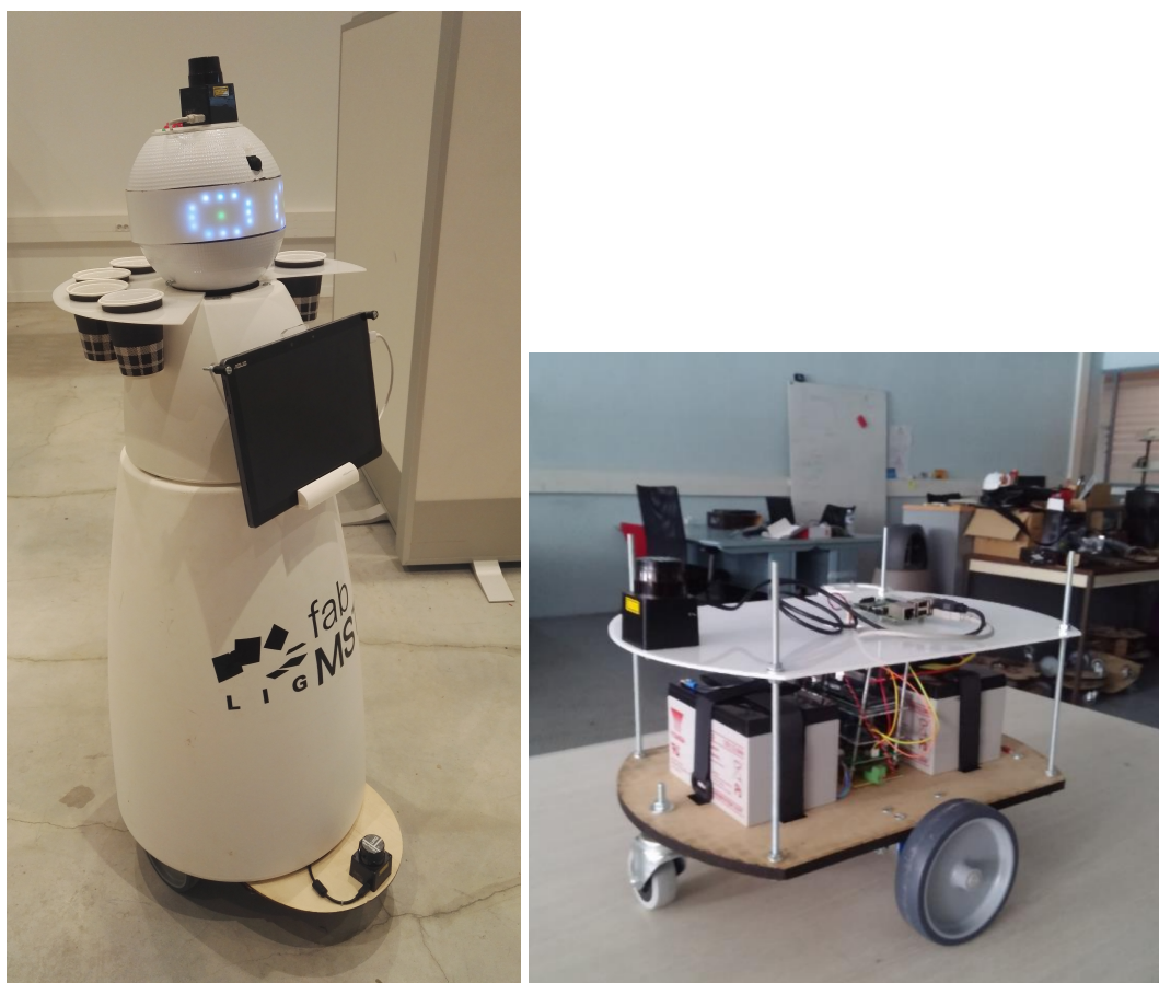
Figure 3.1: Left: RobAIR mobile robot. Right: RobAIR base.
