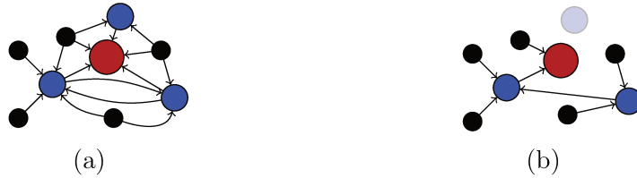
Figure 5.1: Example of a measurements graph \mathcal{G} (a) and a possible IAB Tree \mathcal{T} (b). IAB-donors are depicted in red, IAB-nodes that are not donors in blue, and UEs in black.
