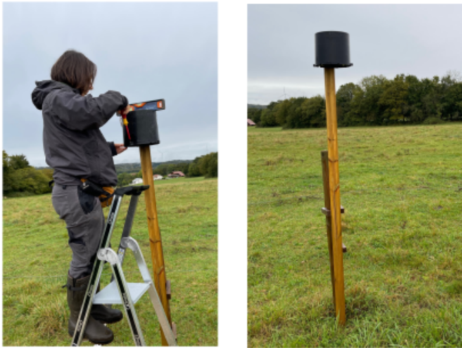
Fig. 2.23 Maintenance and deployment of a rain gauge.
