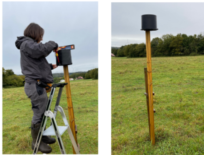
Fig. 2.23 Maintenance and deployment of a rain gauge.
