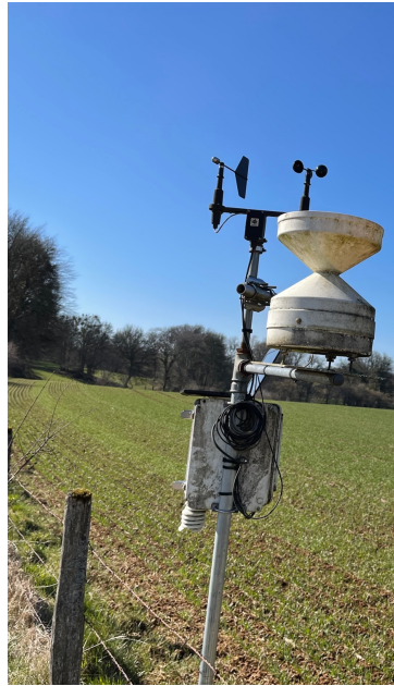
Fig. 2.13 Meteorological station deployed at Fontenotte (SNO Karst).
