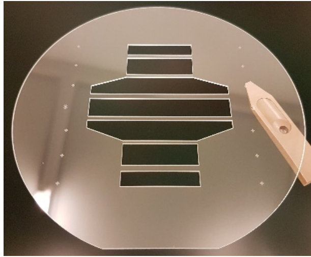
Figure III.4: Glass wafer wet etched by KOH assisted by femtosecond laser
