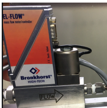
Figure IV.4: Mass flow meter for the flow rate measurement and control in steady flow configuration
