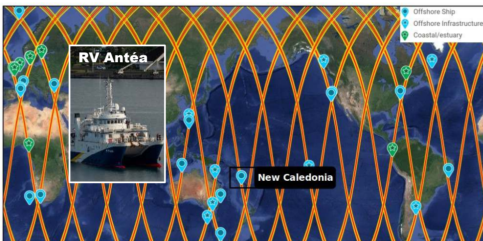
Figure I.30: SWOT fast-sampling phase 1-day repeat orbit. The participating field campaigns (offshore and coastal/estuary) as well observational infrastructure in the framework of the SWOT-AdAC consortium are also shown (adapted from https://www.swot-adac.org/science/ ). The SWOTALIS in-situ experiment south of New Caledonia was carried out in spring 2023 aboard RV Antéa (inset, Credits: J.-M. Bore, IRD)
