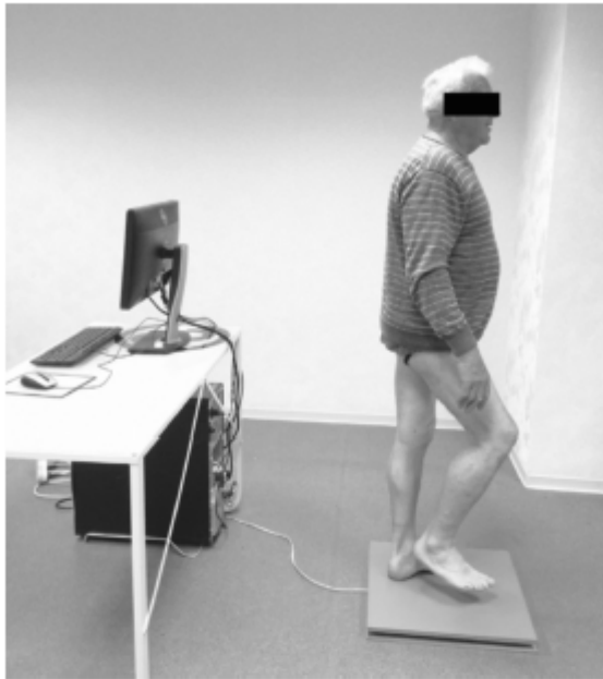
Fig. 2. Stabilometric assessment system: example of a unipedal balance test. Subjects step onto the platform barefoot and stand, quietly, with their knees extended and arms along their sides, looking at a visual marker (red cross) placed on the wall 2 m away.
