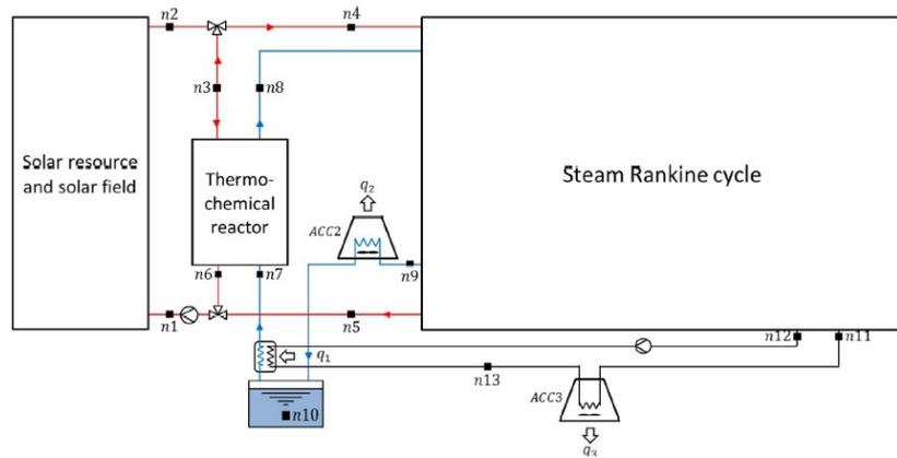
Figure 5.7: Thermochemical storage system. Schema in Storage-Production phase. Copied from [124].
