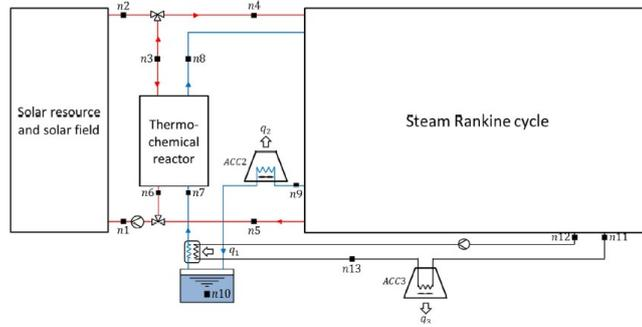
Figure 5.5: Concentrated Solar power plant with Thermochemical storage, including the thermal integration (original Figure from [124]).
