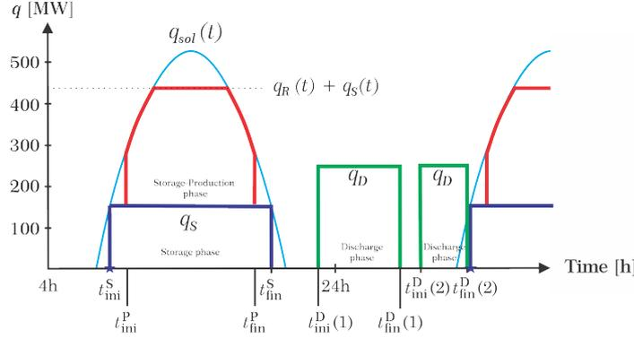
Figure 5.1: Example of a Pre-scenario for one day, one Storage phase, one Storage-Production phase and two Discharges phases.
