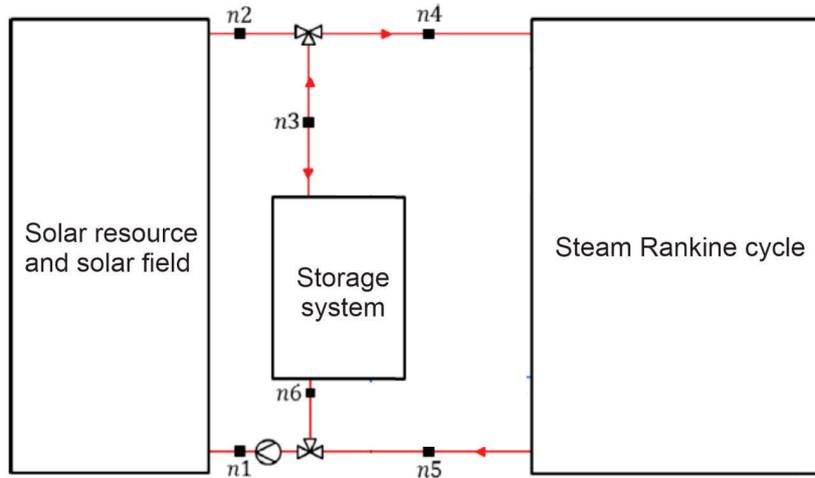
Figure 4.2: Scheme of the black-box model for a Concentrated Solar Power plant. The red circuit represents the main heat-transfer loop.
