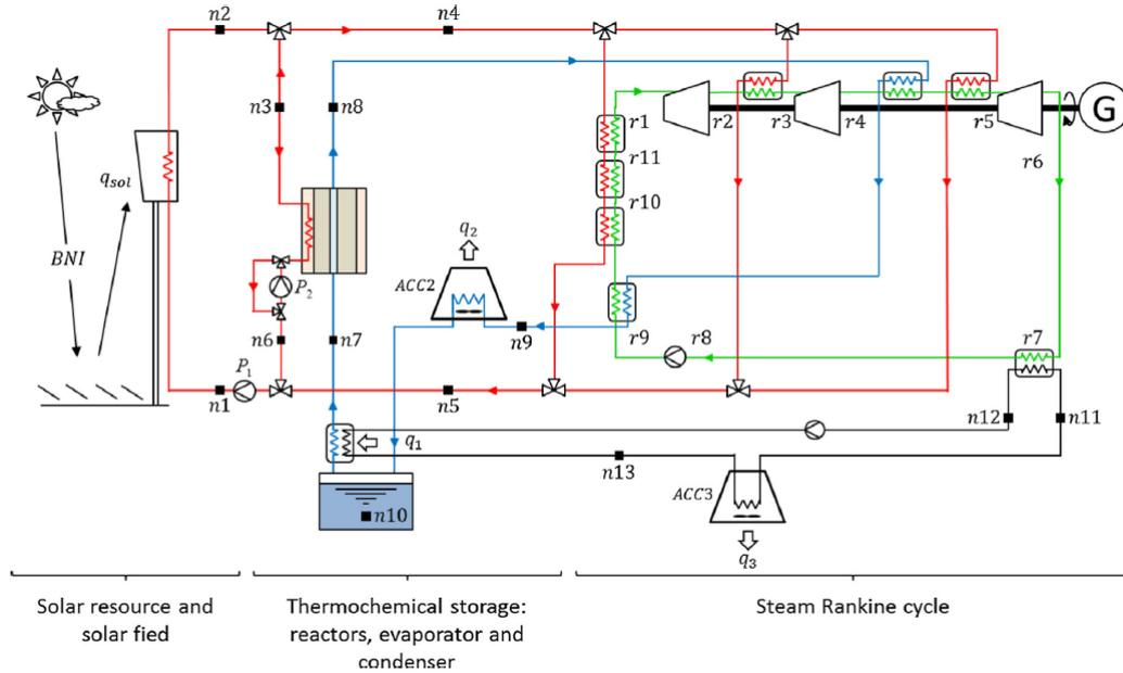
Figure 4.6: Concentrated Solar Power Plan with thermochemical storage.
