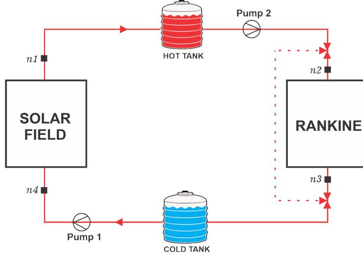
Figure 6.1: Scheme of a CSP plant reduced model.
