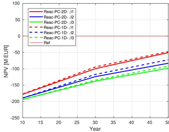
Figure 5.19: Thermochemical system, Price Chasing strategy with one and two Discharge phases, different values for cost parameter  $\beta$ ,  $SM = 2.5$ ,  $\iota_r = 3\%$  and PP scenario.
