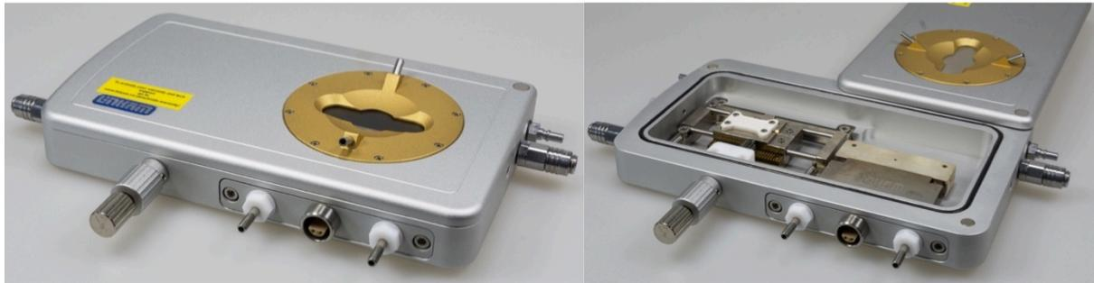
Figure 18 : Cellule Linkam capillaire (Linkam Scientific Instrument Ltd, UK).
