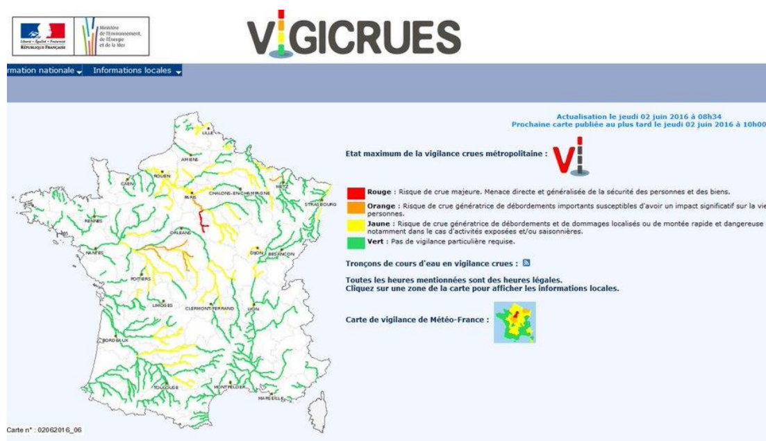
Figure 2-9. Example of river stages monitoring information and flood alert provided on Vigicrues website. (source: Gouvernement (2016)) The red, orange, yellow and green colours show different levels of risk of the rivers: red is the highest and green is the lowest.
