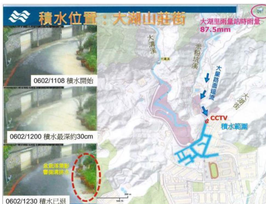
Figure 4-31. The flooded areas (the sky blue areas) and the blocked inlets (the red dashed circle). (source: Taipei City Fire Department (2017a)) The peak accumulated rainfall in an hour recorded by a rain gauge at the upper right corner of the figure was 87.5 mm. According to the videos from the CCTV, the flood started at 11:08 on June 2, with the maximum water depth reaching about 30 centimetres at 12:00, and the flood receded at 12:30.
