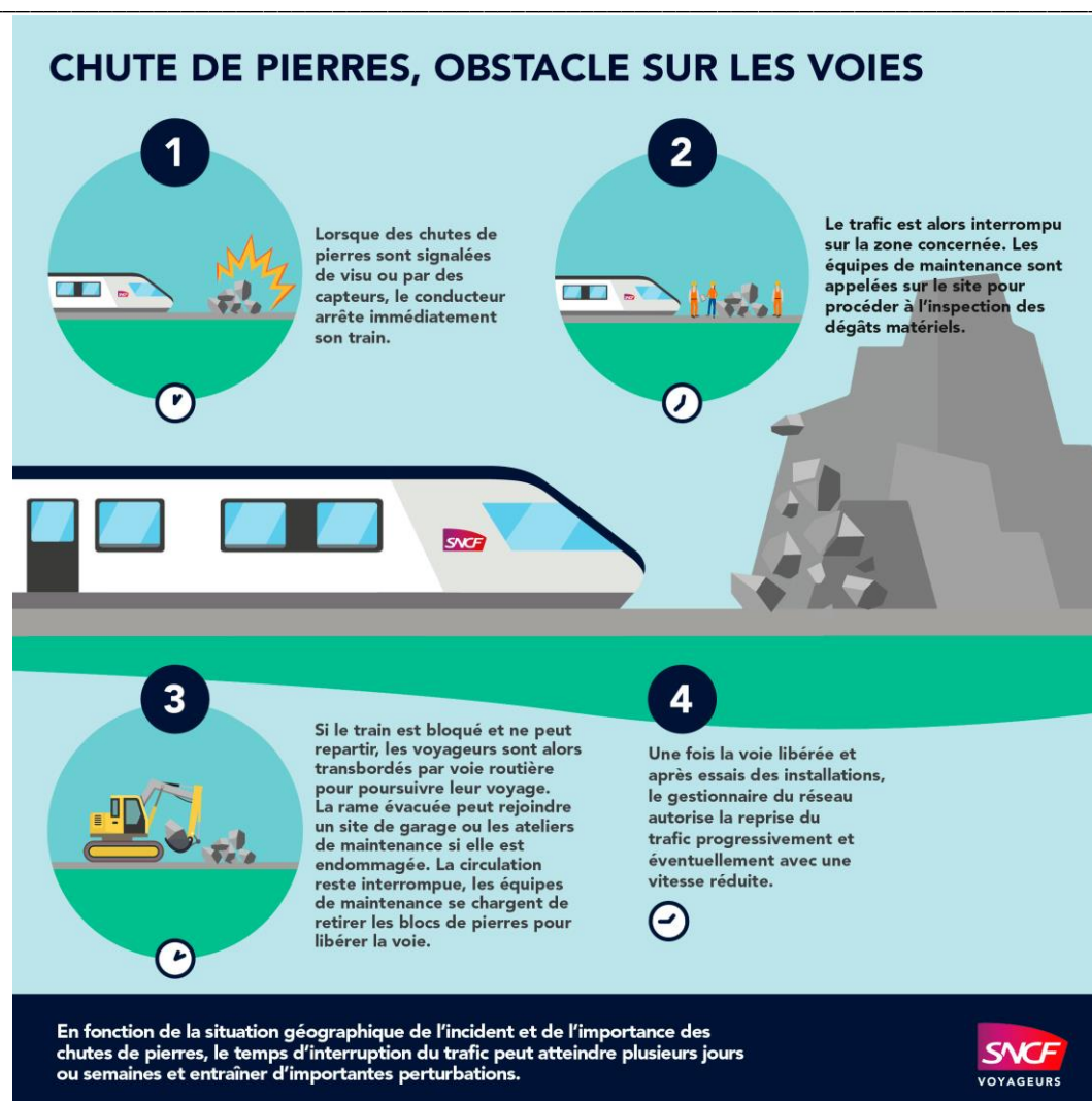
Figure 2-15. Train traffic was interrupted after a rock falls on the railway track. (source: SNCF (2023)) The texts in French mean: 1. When rockfalls are signalled visually or by sensors, the driver immediately stops the train; 2. The traffic will be interrupted in the concerned area. Then, maintenance teams will be called to the site to inspect the material damage. 3. If the train is blocked and cannot leave, passengers will be transferred by road transport. The evacuated train can reach a garage site or the maintenance workshops if it is damaged. If traffic remains interrupted, the maintenance teams are responsible for removing the rocks to free the track. 4. Once the track has been freed and after installation tests, the network manager authorises the resumption of traffic gradually and possibly at a reduced speed
