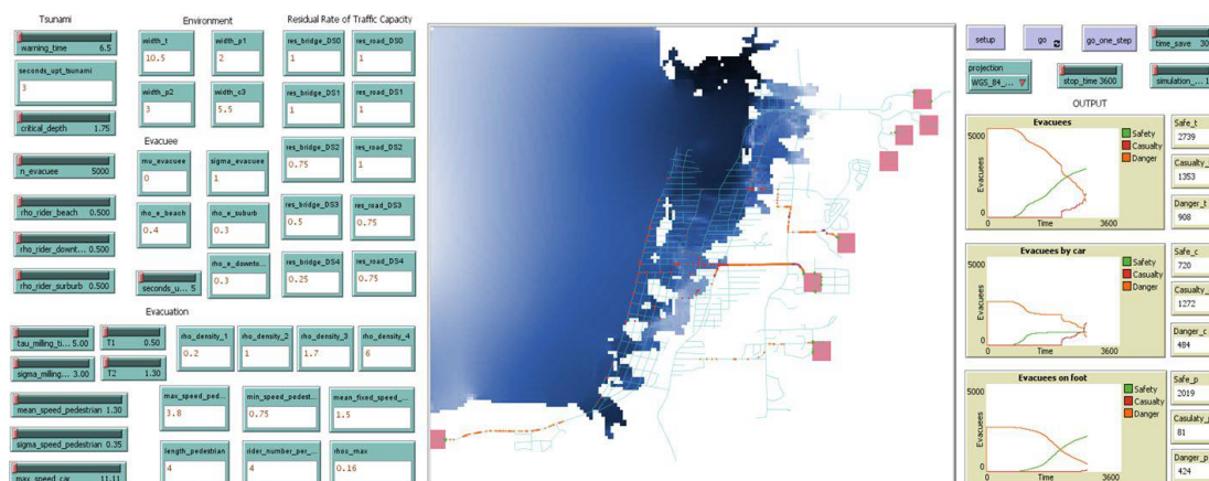
Figure 2-24. A screenshot of the agent-based tsunami evacuation model. (source: Wang & Jia (2021))
