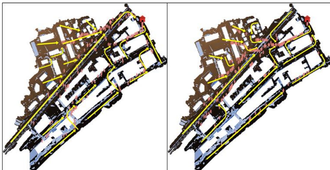
Figure 4-6. The general evacuation routes chosen by evacuees without (left) and with (right) the consideration of risk maps and flood maps.
