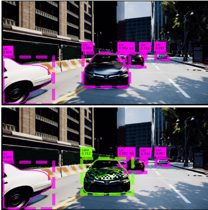
FIGURE 1.7: The camouflage fools the Mask R-CNN object detector (on the bottom), whereas plain colours (on top) are being correctly detected [130].
