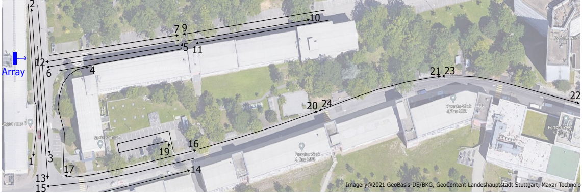
Figure 2.8: Image of the Nokia campus in Stuttgart, Germany. The transmit array's location (resp. boresight direction) is marked on the left by a blue bar (resp. blue arrow). The measurement tracks along which the vehicle (mimicking a UE) was moved are depicted by black lines. The corresponding arrowheads and numbers indicate the direction of movement and the measurement track number. Source: [2].
