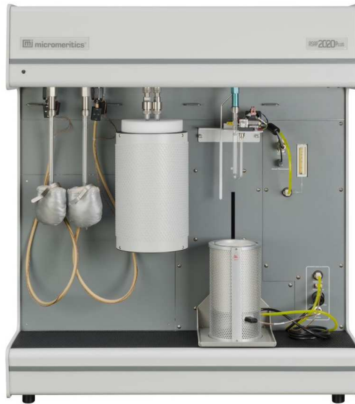
Figure A9: Image obtained from Ref. [375] showing the Micromeritics ASAP200 apparatus used for the nitrogen sorption experiments.
