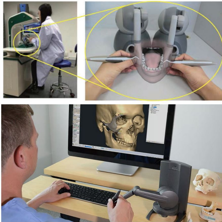
Figure 1.12: Examples of grounded haptic devices. Starting from the top: Dentist during training with VOXEL-MAN Virtual Dental Training Simulator [47], TouchX series from 3D System Inc. [48]
