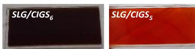
**Figure 9: The deposited CIGS<sub>6</sub> and CIG<sub>5</sub> samples on soda lime glass.**
