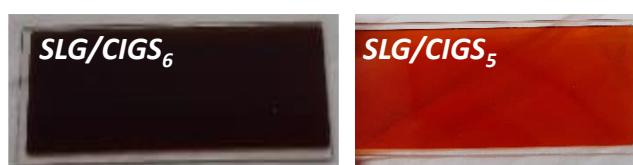
Figure 9: The deposited CIGS 6 and CIG 5 samples on soda lime glass.
