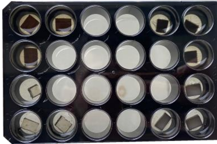
Figure 80: 24-well microtiter glass bottom plate. Microorganisms adhesion takes place in the well containing a material sample. Empty spots are used to flip the samples and analyze the covering surface by confocal analysis.
