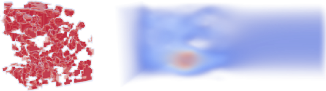
Figure 5.20: Solid soot domain (left) and stationary solution of the velocity magnitude (right) for the mass conservation test case.
