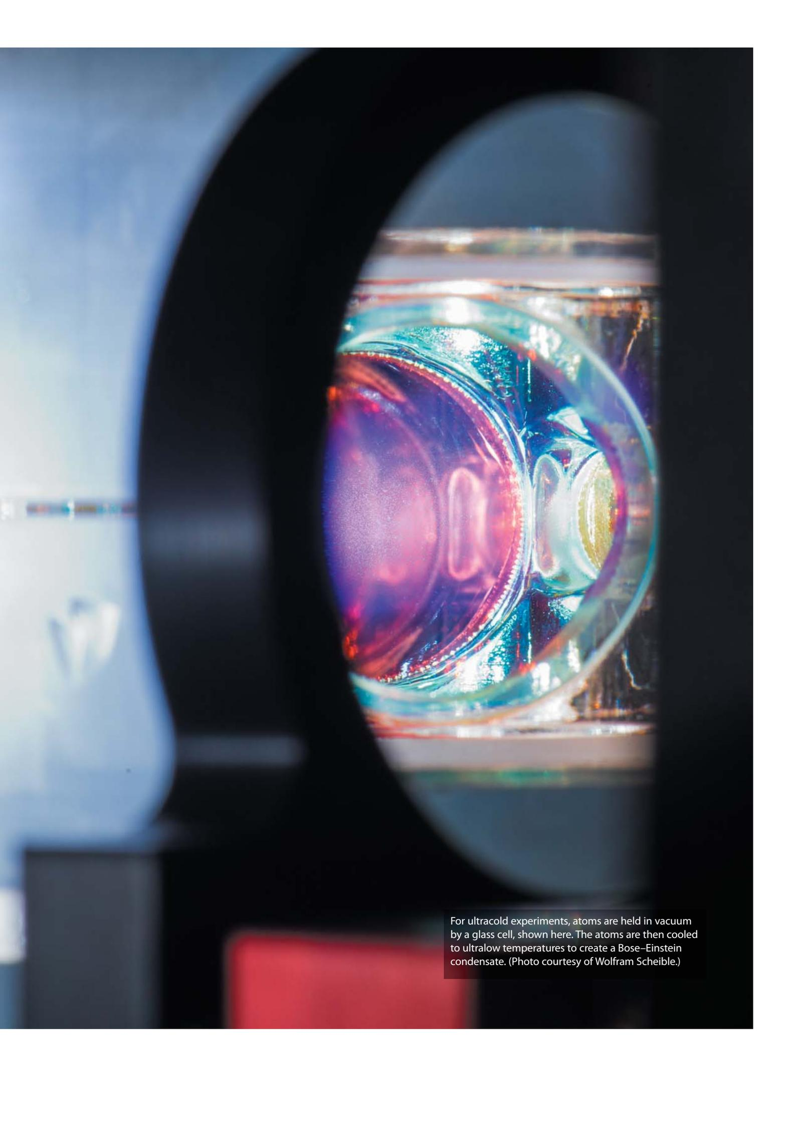
For ultracold experiments, atoms are held in vacuum by a glass cell, shown here. The atoms are then cooled to ultralow temperatures to create a Bose–Einstein condensate. (Photo courtesy of Wolfram Scheible.)
