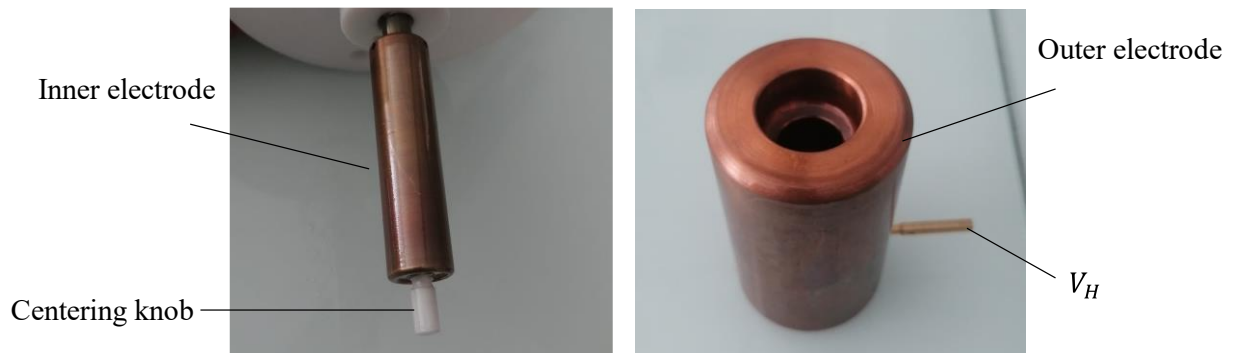
Fig 4.2. Inner and outer concentric copper electrodes used for EHD heat transfer enhancement studies in dielectric liquid
