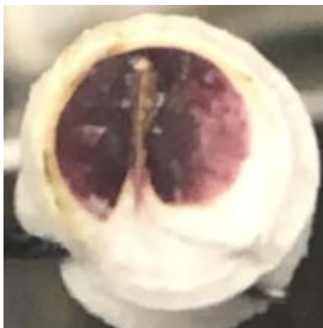
Figure S60. Picture of the used separator, showing the purple compound, after a galvanostatic discharge experiment.
