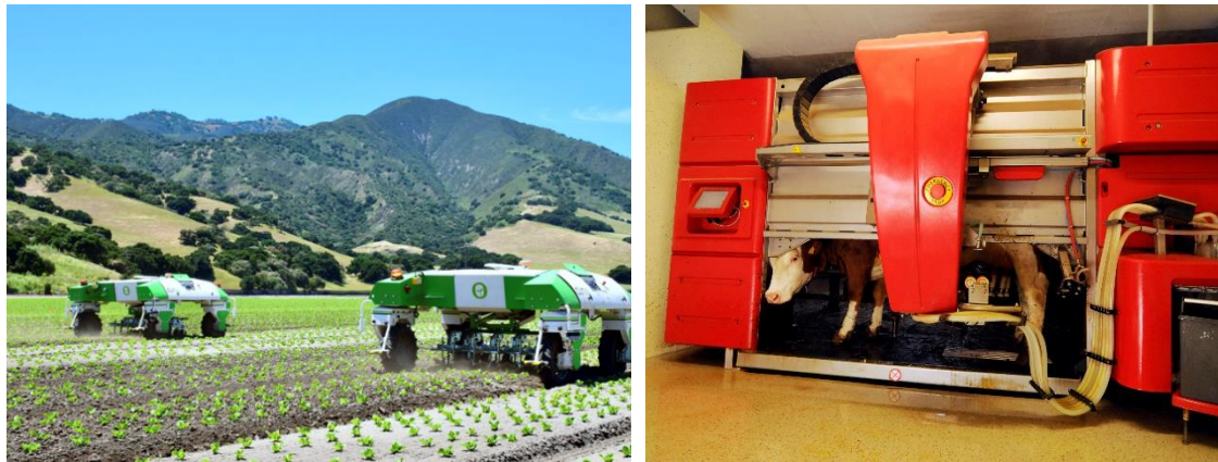
Figure 12 : left: weeding robot for vegetable production, photo by Naïo Technologie; right: automated milking system, iStock photo by Elmar Gubisch
