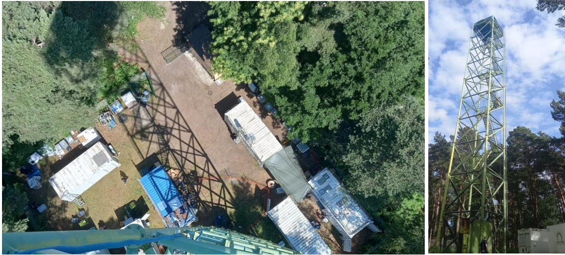
Figure 4.1. Photos of the measurement site in the Rambouillet Forest (from the top of the tower on the left) and a view of the 40-m tower (on the right) during the ACROSS summer campaign.
