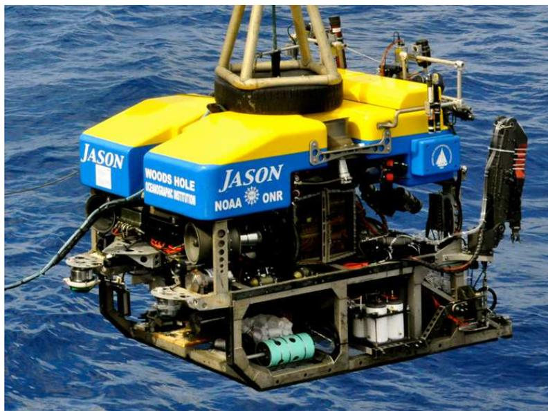
Figure 1.2: Jason ROV of the Woods Hole Oceanographic Institution / National Ocean and Atmospheric Administration, about to be deployed from a crane. Image source: [116]
