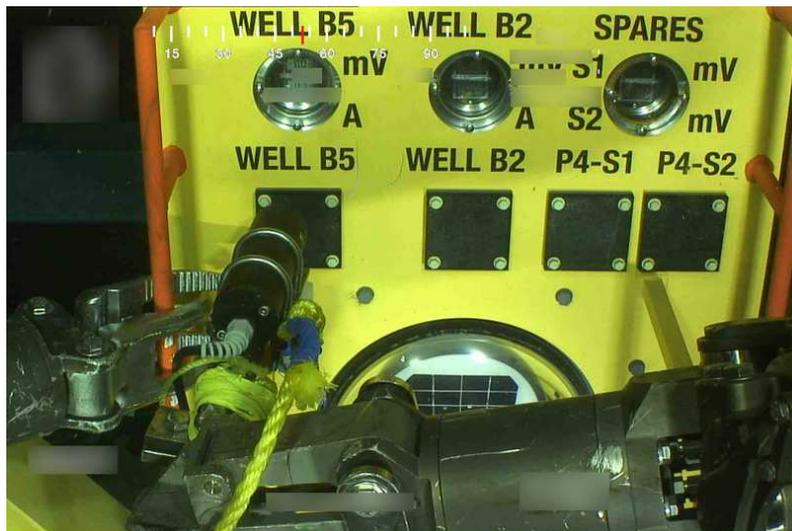
Figure 1.15: This could be the view from the on-board camera of the ROV from the previous picture. The yellow panel equipped with brown grab-bars presents a good planar target with characteristic patterns and high contrasts. Most of subsea oil field structures follow this sort of painting scheme. Image source: [135].
