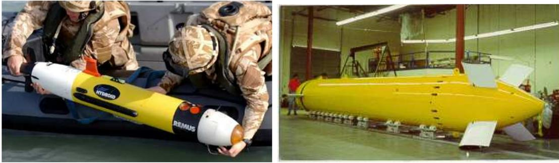
Figure 1.4: From the smallest to the biggest: Kongsberg's REMUS AUV (image source: [130]) at 1.60m and 40kg and ISE's THESEUS cable-laying AUV (image source: [131]) at 10.70m and 8,600kg (each of the control fins is longer than 1m). Both are torpedo-shaped, underactuated AUVs.
