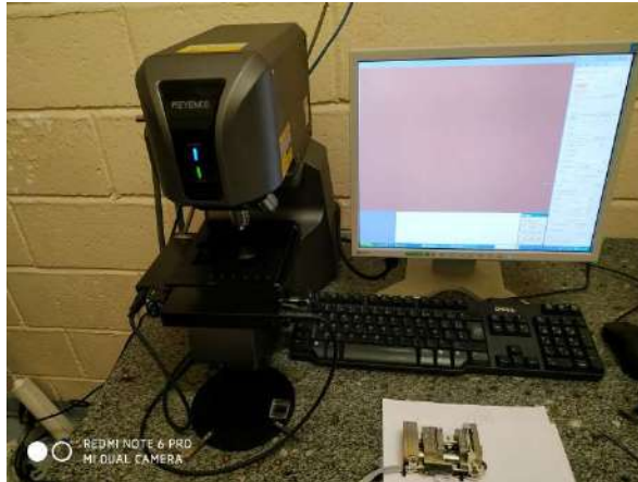
Figure 2.25 – KEYENCE confocal microscope coupled to the micro-tensile test DEBEN device.
