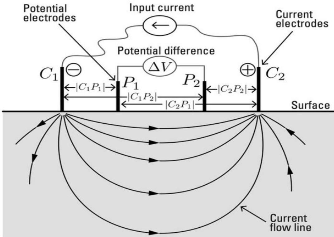
Figure 2. 1: Quadripolar configuration in a homogeneous half space showing current flow.  $C_1$ ,  $C_2$  represent electrodes pushing current into the subsurface and  $P_1$ ,  $P_2$  denote potential electrodes (Conti et al., 2021) for measuring potential difference.
