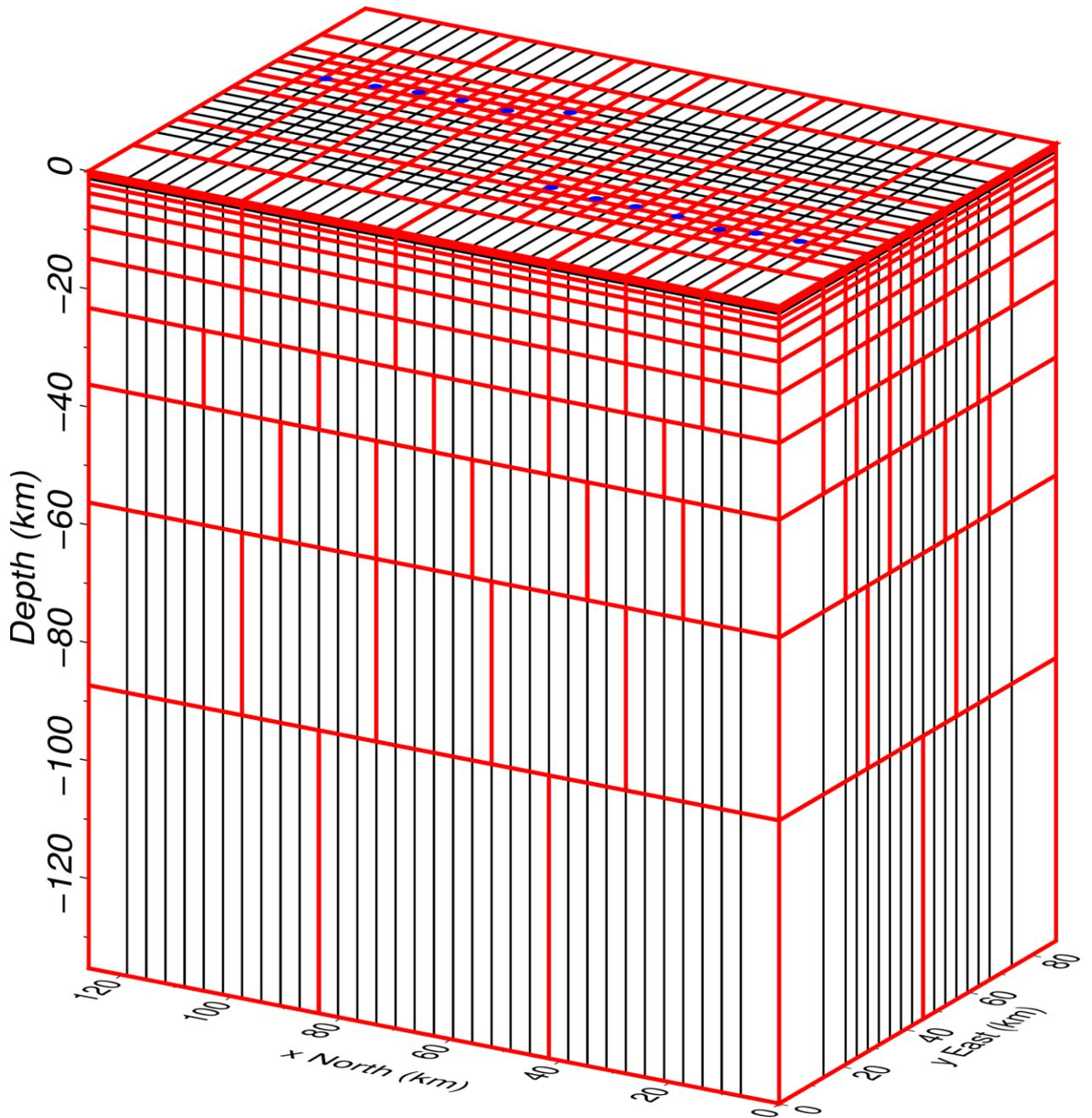
Supplementary Figure 2: 3D model grid. Blue dots on the plan view represent MT stations
