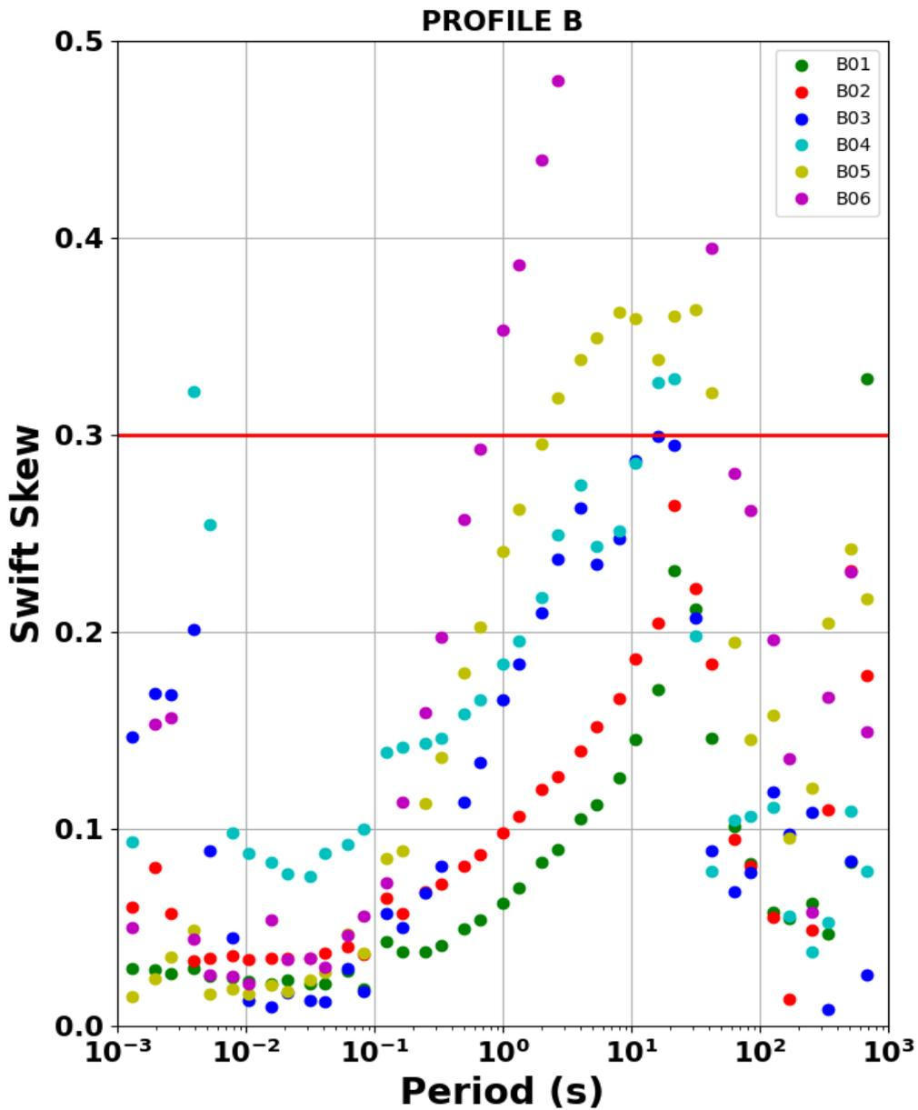
Figure 7. 5: Swift skew values for all sites with different colors representing different MT sounding stations shown in legend of the graphs. (a) most sites in profile A plotted below 0.3 threshold (red solid line) at short periods (b) shows all sites along profile B with majority of skew values plotting below 0.3 indicating 1-D or 2-D structure. 3-D structure is observed at long periods shown few skew values plotting above 0.3 for both profiles.
