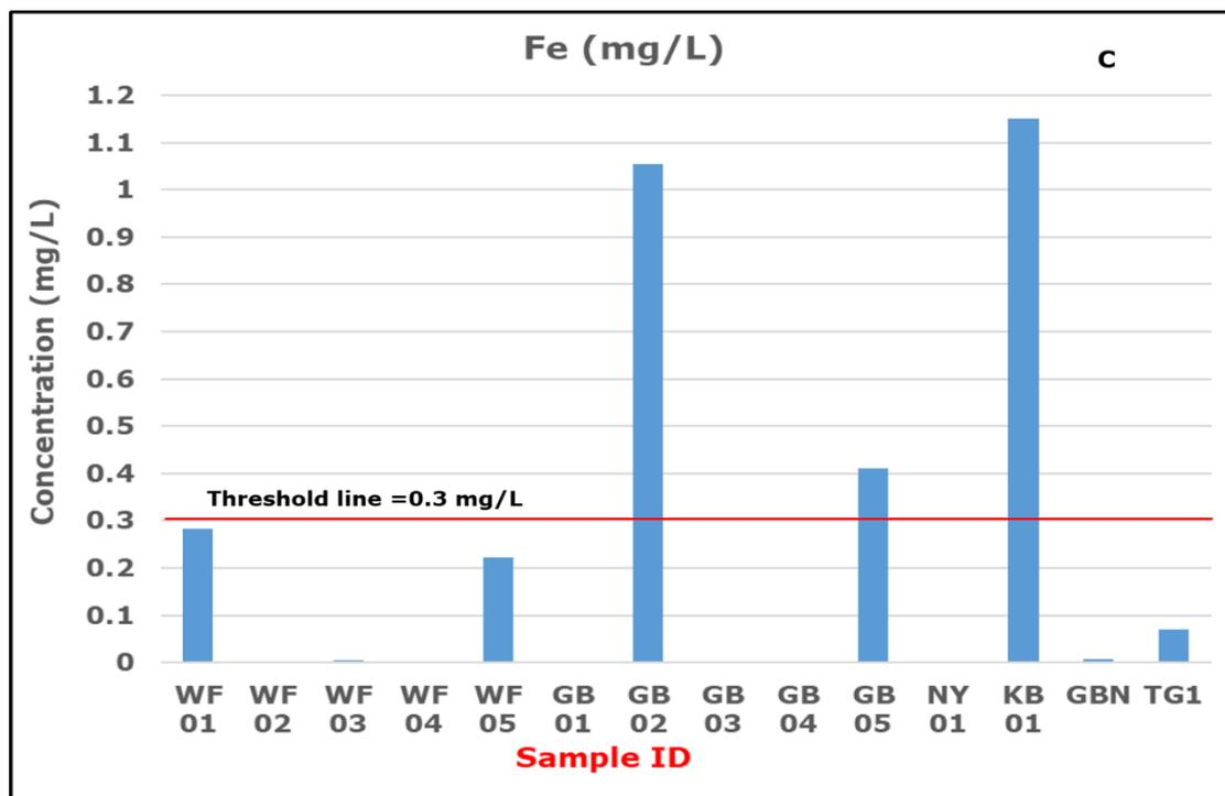
Figure 4. 7: Plots of heavy metals concentration verse sample ID showing which metal in which sample exceeds the recommended threshold values as suggested by GEPA and WHO. (a) is plot for Pb, Zn, Cr, Cu (b) is a plot Cd and (b) is a plot of Fe concentrations.
