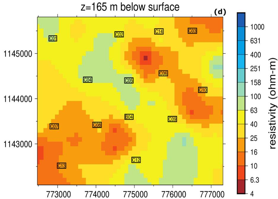
Figure 6. 6: Horizontal depth slices showing of 3-D resistivity model: (a) potential saprock aquifer trending NE-SW (b) NW-SE paleovalley at 50m identified by erstwhile Dzikunoo et al. (2020) connect to extended network of fractures forming a potential peripheral aquifer (c) NW-SE paleovalley at ~94m (d) potential groundwater productive unit formed from network of fractures at 165m deep.
