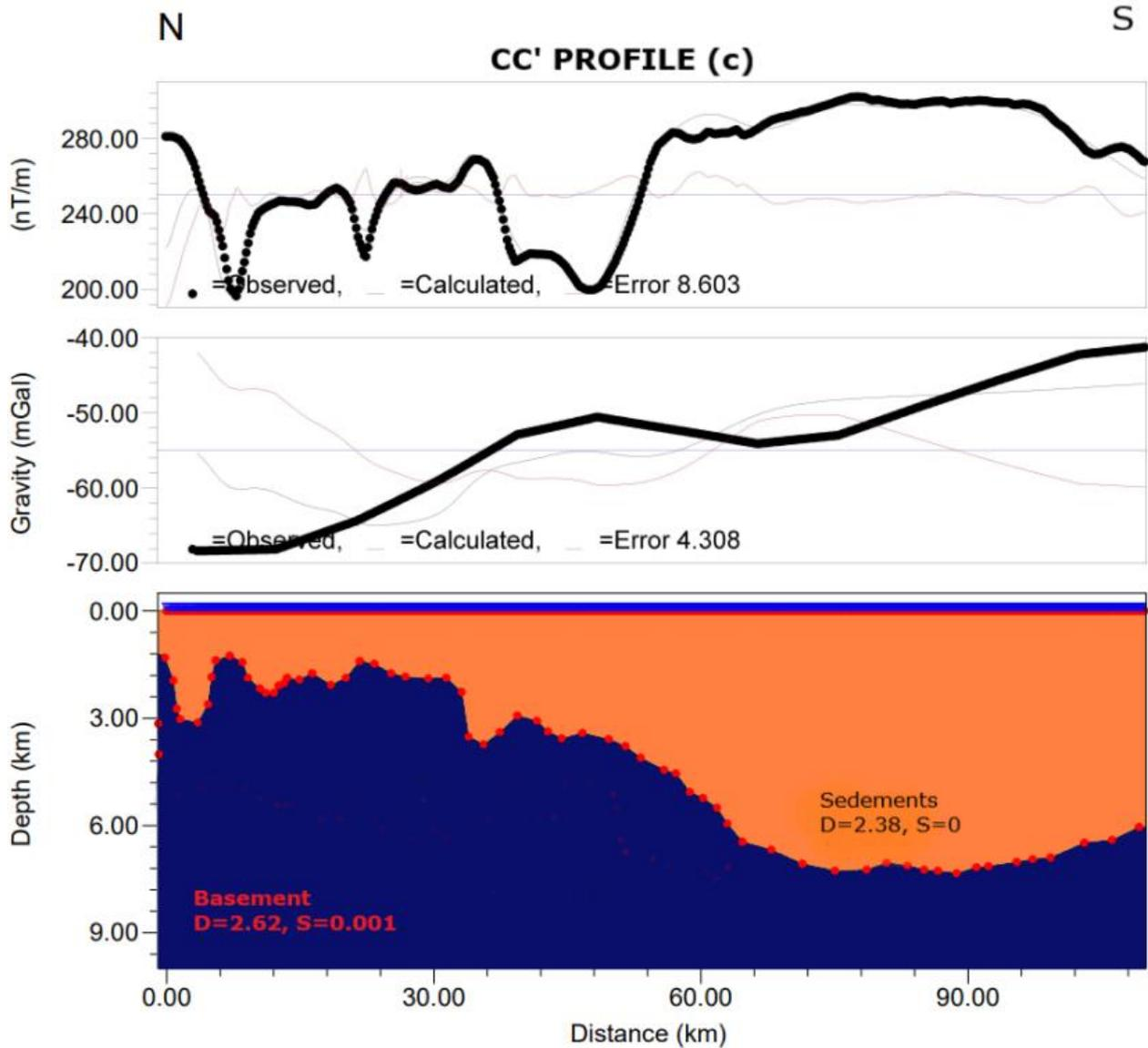
Figure 7. 4: 2-D models of aerogravity and aeromagnetic data showing sediment-basement boundary and morphology of the basement along three NS profiles: (a) AA<sup>1</sup> Profile, (b) BB<sup>1</sup> Profile and (c) CC<sup>1</sup> Profile.
