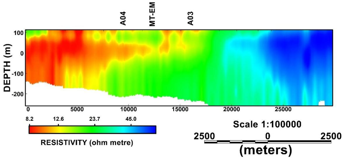
Supplementary Figure 5: 2-D cross-sections along AEM flight lines showing variation in resistivity representing geological variations in the study area. The sections were plotted using the Oasis Montaj program in geosoft.
