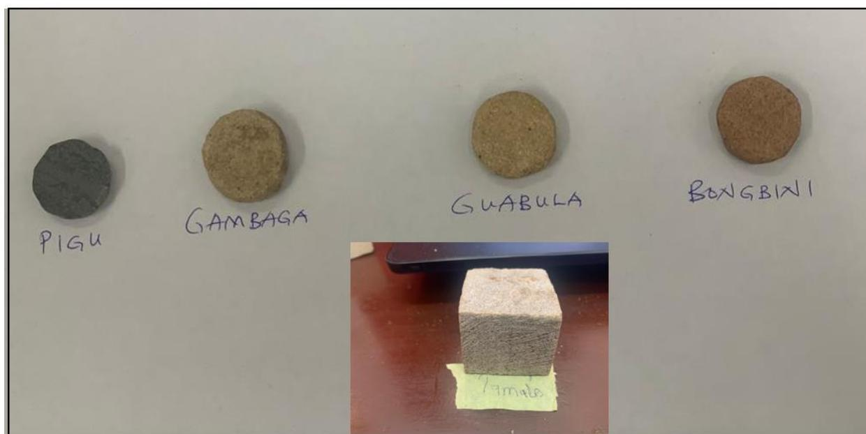
Figure 3. 3: Rock samples prepared for SEM-EDX Analysis. Each of the five samples analyzed are shown in the image.
