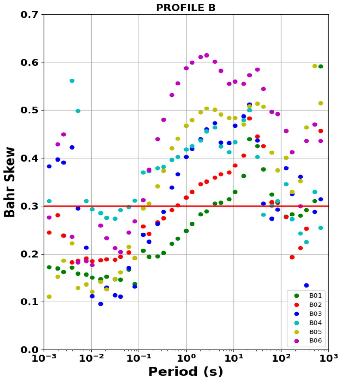
Figure 7. 6: Bahr skew values of all sites represented by different colors; (a) most of the sites along profile A plotted below 0.3 suggesting a 1-D or 2-D structure at short periods while a significant number of the values plotted above 0.3 indicating a 3-D structure present. (b) few sites are plotted below 0.3 at short periods whilst to most sites plotted above 0.3 at long periods indicating a 3-D subsurface structure.
