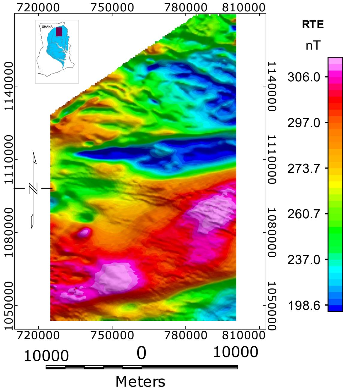
Supplementary Figure 1: Reduced to the Equator showing magnetic anomalies: red represents high magnetic intensity anomaly and blue represents low magnetic anomaly.
