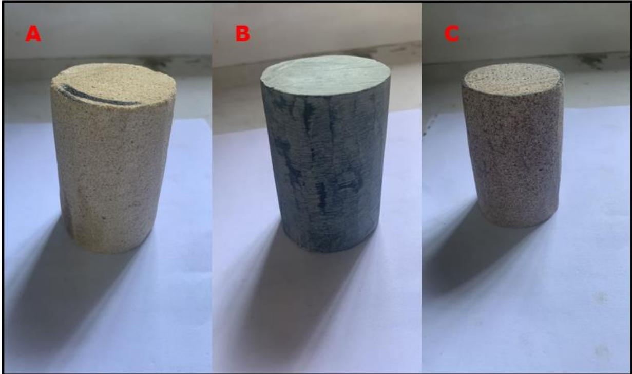
Figure 3. 2: Field samples being prepared for thin sections and SEM analysis; (a) Panabako sandstone north of profile B (b) Carbonate rock south of profile B and close to MT station A01 and (c) Tamale sandstone south of profile A.
