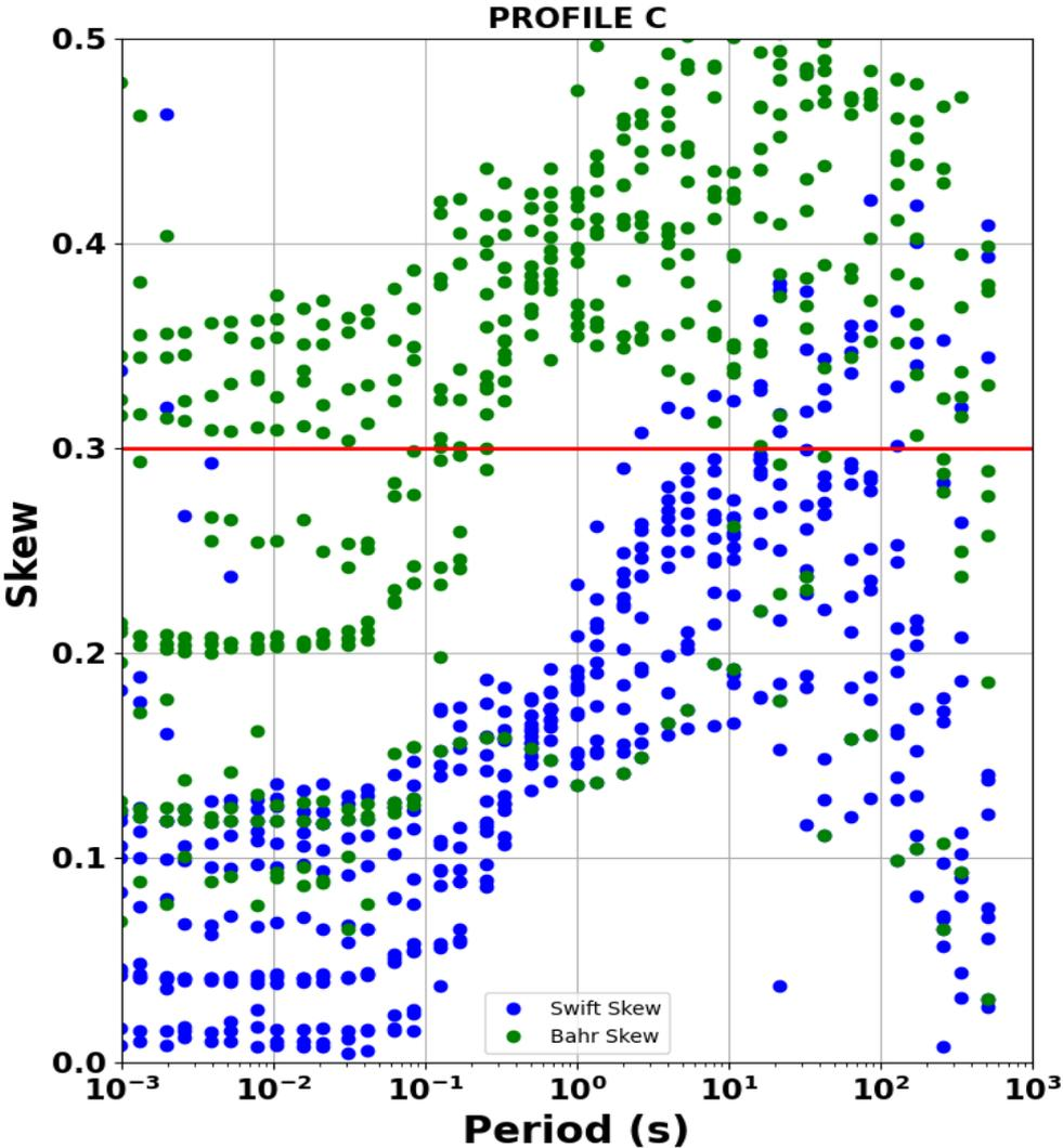
Figure 6. 3: A plot showing skewness as a measure of dimensionality of the MT data. Red straight line indicates the threshold for the determination of dimensionality. Blue and green dots represent Swift and Bahr skew respectively.
