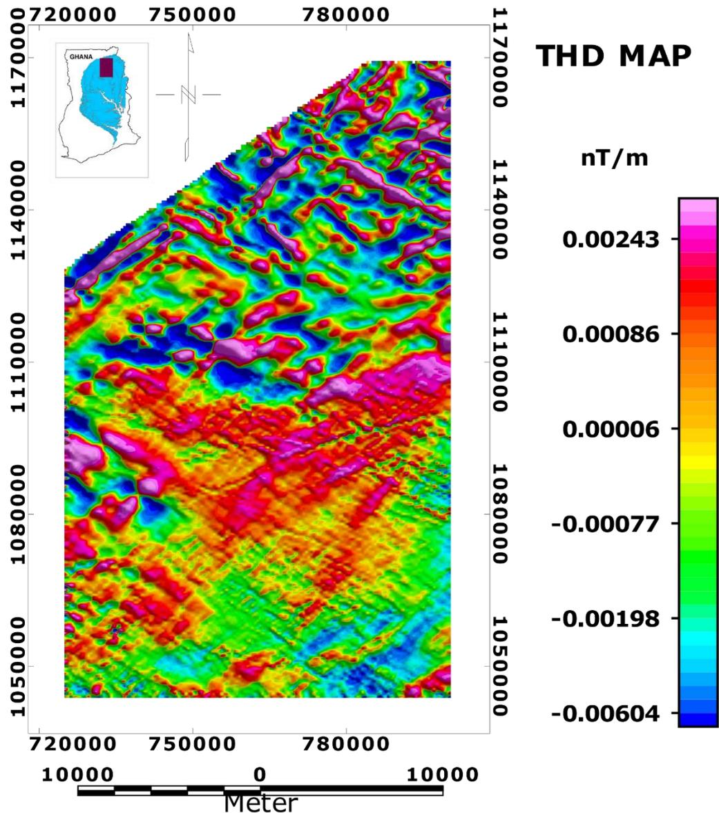
Figure 5. 3: Total horizontal derivative maps showing variational direction of linear structure with inset map of Ghana showing coverage of the VSB and location the current study.
