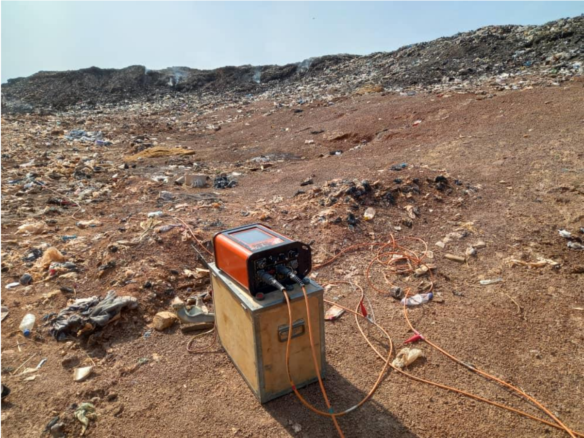
Figure 2. 6: Field setup using the ABEM LS Terrameter at Taha dumpsite located in the Tamale metropolitan district, northern Ghana.
