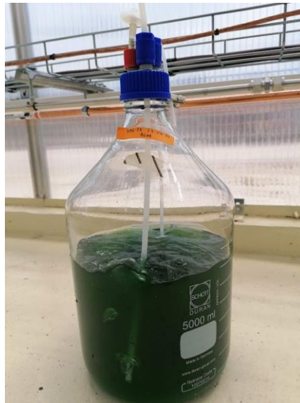
Figure 30 Experimental device to characterize the CO 2 assimilation in a 3 L system
