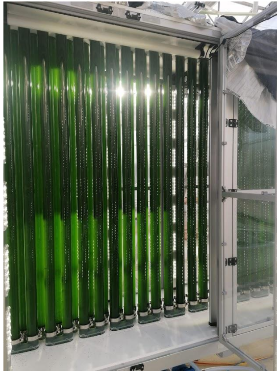
Figure 38 Tubular photobioreactor (JUMBO, Synoxis Algae, France) employed for the biomass production for extraction tests
