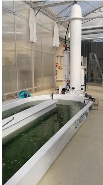
Figure 31 3 m 3 Raceway Coldep system
