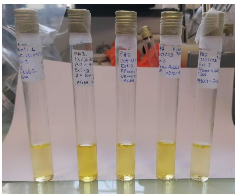
Figure 93 Supercritical CO 2 extraction at 300 bar and 60°C extract from Arthrospira platensis , suspended in 5mL of ethanol.
