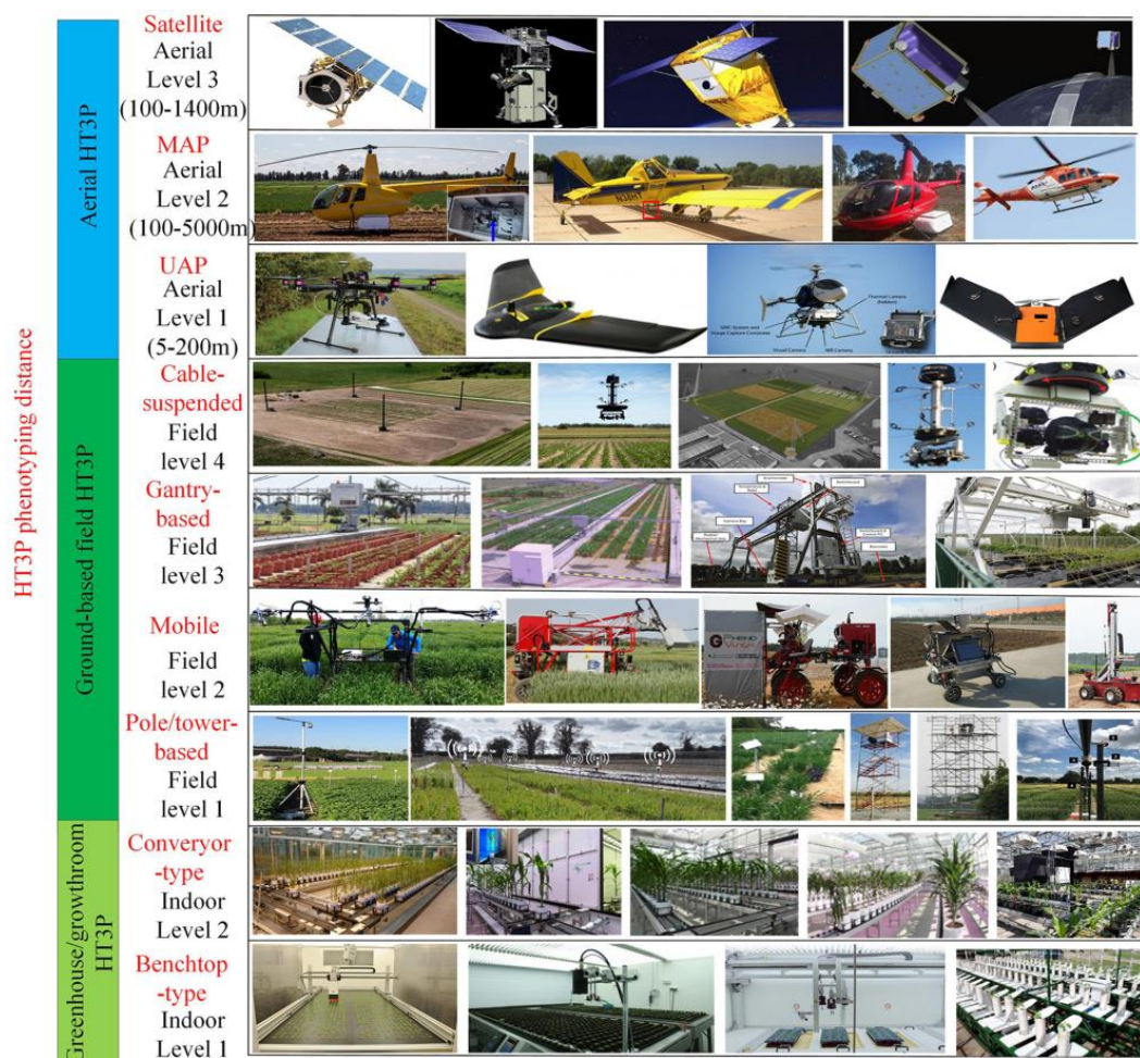
Fig. 5 : Examples of high-throughput plant phenotyping platforms (HT3Ps) as reviewed by Li et al., (2021), including HT3Ps in the greenhouse/growth chamber, field ground-based HT3Ps and aerial HT3Ps.
