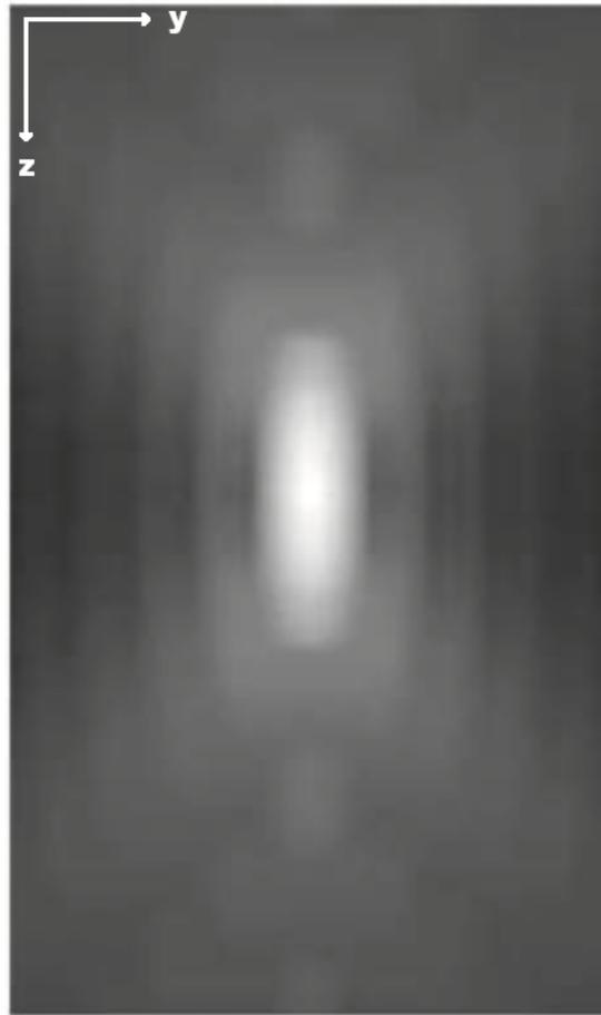
Figure 1.10 – Simulation of the PSF generated by a microscope with  $\lambda = 557 \text{ nm}$  and  $\text{NA} = 1.3$ , as observed in the axial plane. To improve the visualization of the diffraction rings, the image was contrasted with a factor  $\gamma = 0.5$ . (illustration extracted and edited from [Cole, Jinadasa, and Brown 2011])
