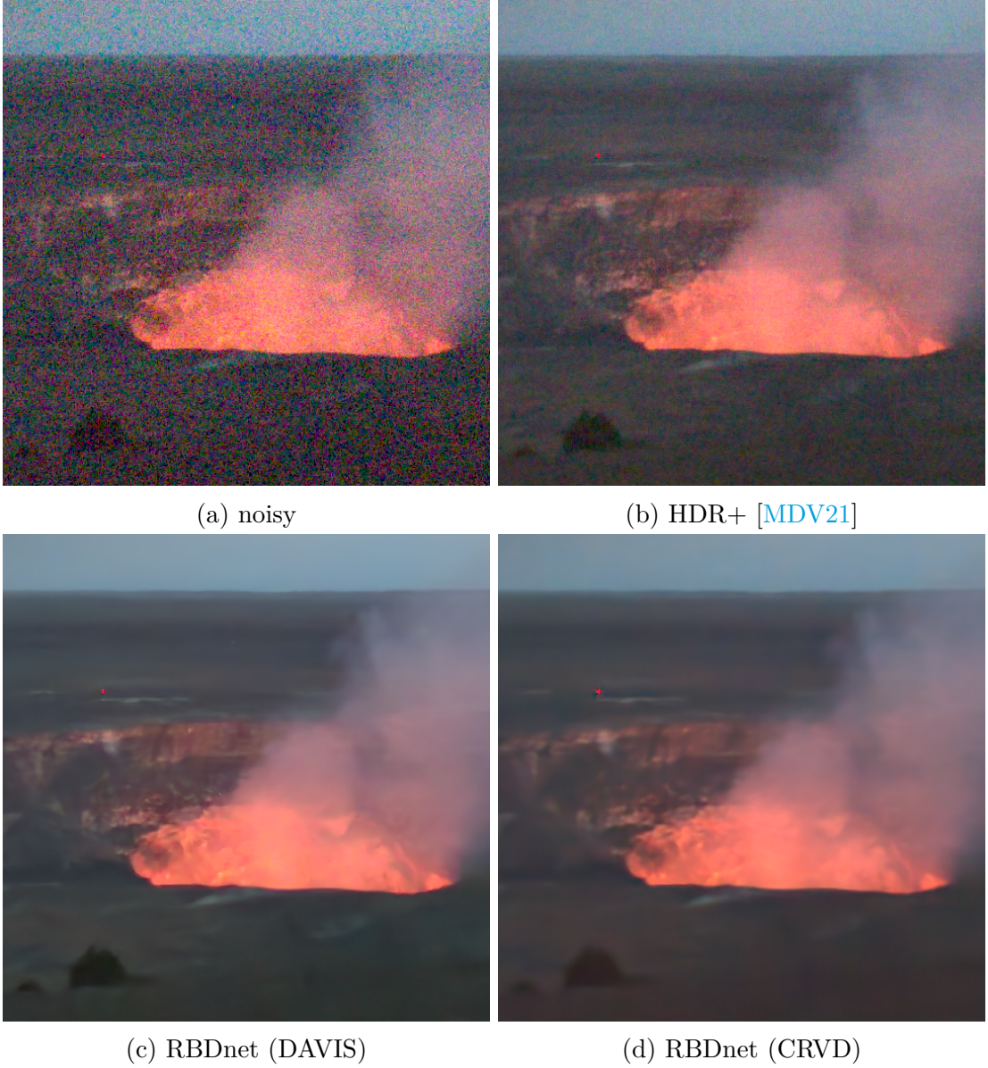
Figure 2.14: Burst denoising of frame 2 of burst 33TJ_20150820_190702_015 (ISO 1877; all models take 5 4208 \times 3120 Bayer frames as input; 540 \times 540 crops are shown here)
