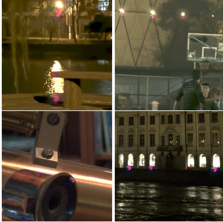
Figure 2.10: Artifacts observed on some bursts after denoising with RBDnet trained on unprocessed DAVIS with per-channel per-frame noise maps.
