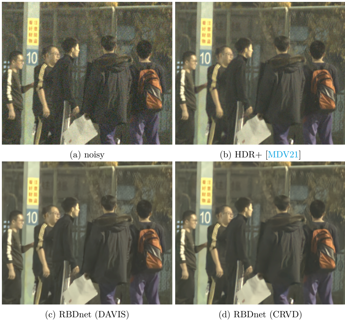
Figure 2.11: Burst denoising of frame 2 of CRVD sequence 4 (ISO 6400; all models take 5 1920 \times 1080 Bayer frames as input; 500 \times 420 crops are shown here)
