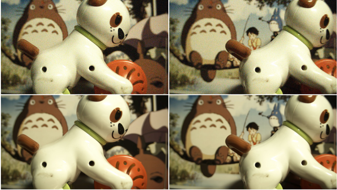
Figure 2.9: 2 consecutive 1920 \times 1080 frames of a CRVD indoor scene at ISO 25600. Top row: noisy images. Second row: clean images. (best viewed digitally; images processed to sRGB for visualization)
