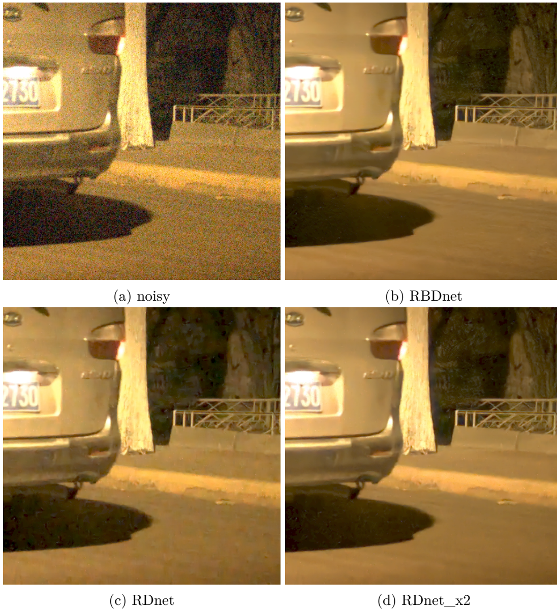
Figure 2.15: Multi-frame vs single-frame denoising of frame 2 of CRVD sequence 1 (ISO 25600; all models are trained on the same DAVIS samples; 480 \times 480 crops are shown here)
