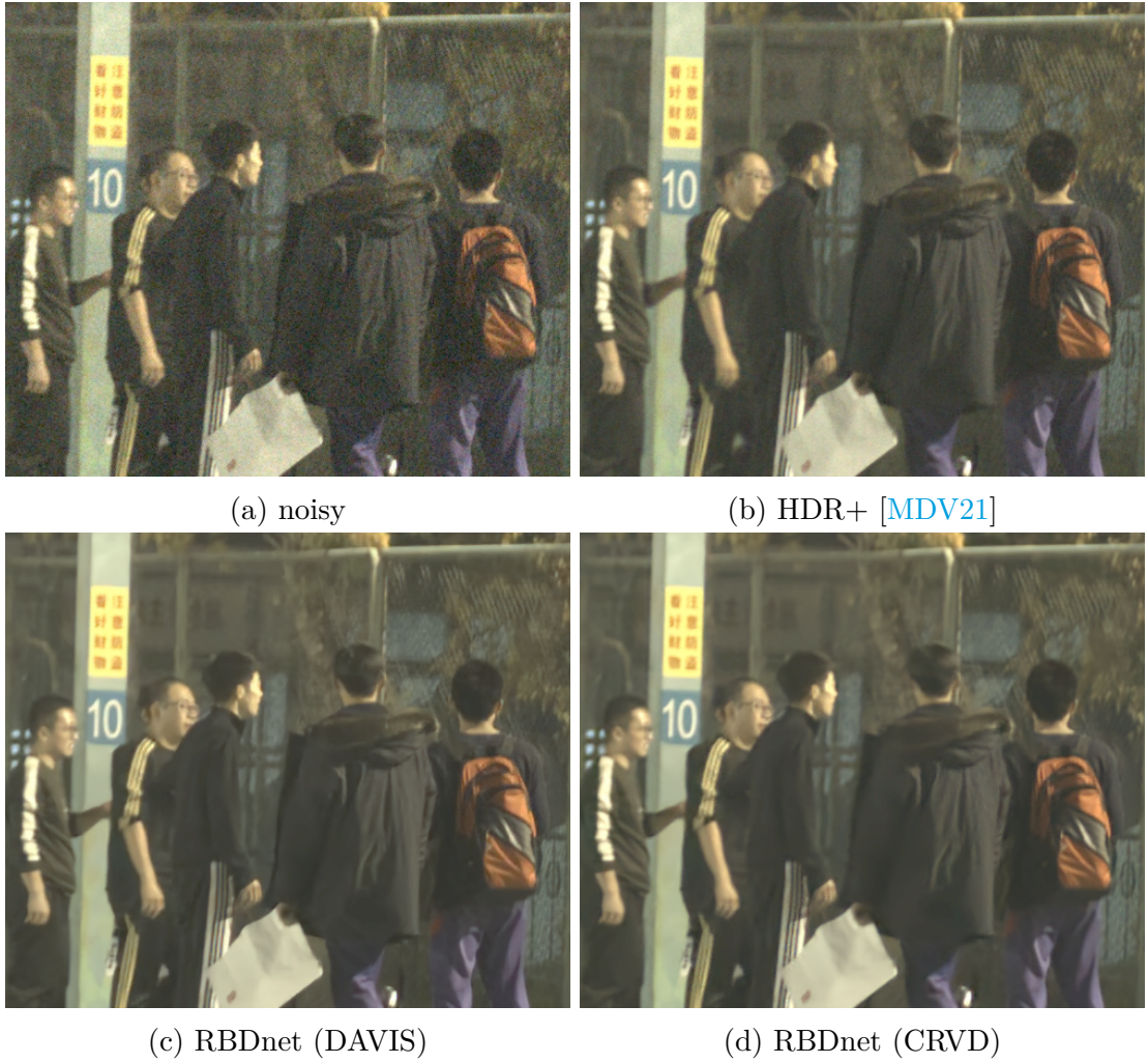
Figure 2.11: Burst denoising of frame 2 of CRVD sequence 4 (ISO 6400; all models take 5 1920 \times 1080 Bayer frames as input; 500 \times 420 crops are shown here)
