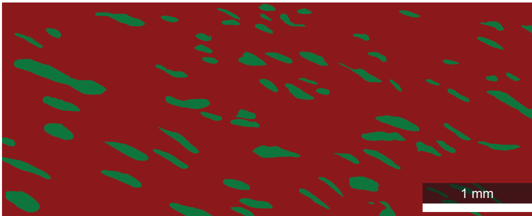
Figure 2.24: SEM stitching from x150 magnification micrographs, differentiation from FG (green) and MG (red) regions
