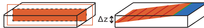
Figure 2.15: Subsurface observation methodologies: left: cross-section cutting and grinding / right: wedge coupon grinding
