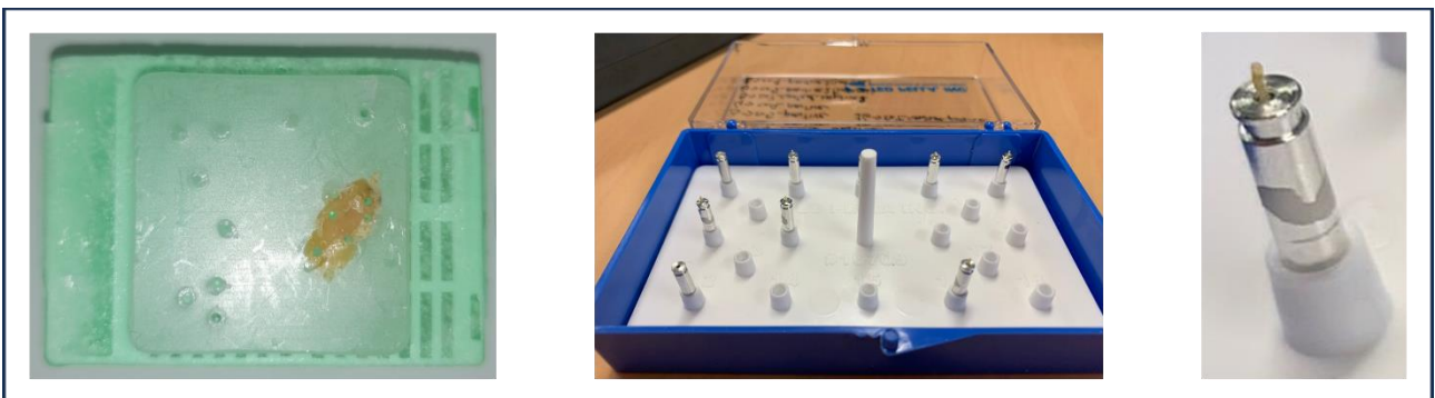
Figure 4.16 Sample preparation pictures. From the left: punched hemibrain embedded in paraffin, samples mounted on metallic pins in a box, detail of the mounted sample.
