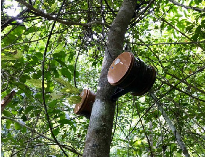
Figure 1.10: Acoustic Sensor for Environmental Monitoring[15].
