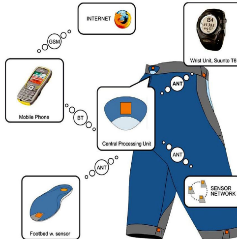
Figure 1.8: Example of Wearable Device with Multiple Sensors[12].
