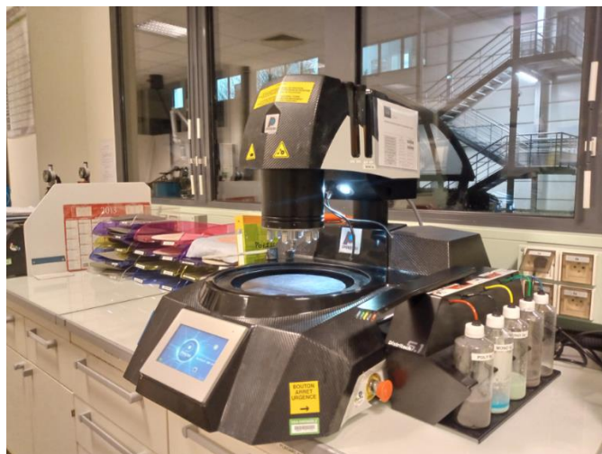
Figure 50: Equipment « Mecatech 300 » by PRESI used for polishing.
