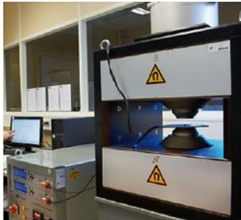
Figure 56 : Hysteresigraph system used at CEA-LITEN for magnetic characterization. Adapted from Fliegans 92 .
