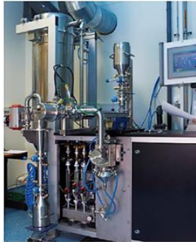
Figure 41 : Nitrogen jet milling device used at CEA/LITEN. Adapted from Fliegans 92 .
