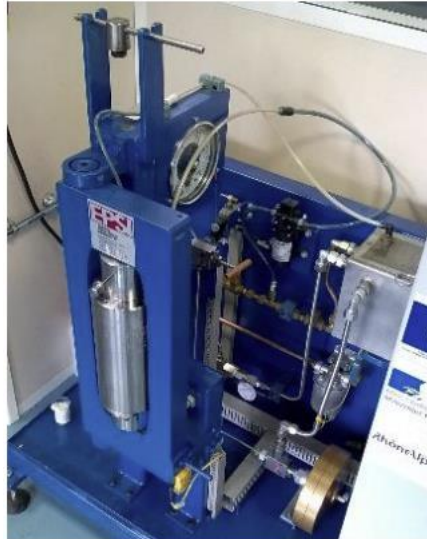
Figure 43: Cold isostatic pressing system used at CEA/LITEN for compressing powders.
