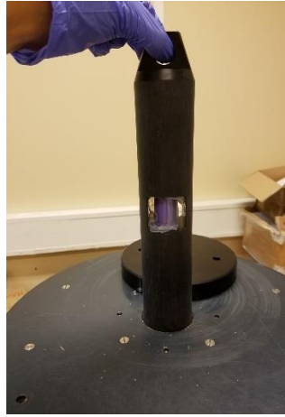
Figure 42: Bitter coil used for magnetic alignment.
