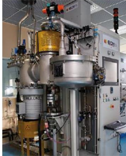
Figure 44: Furnace used at CEA-LITEN for sintering, annealing and diffusion heat treatments. Taken from Fliegans 92 .
