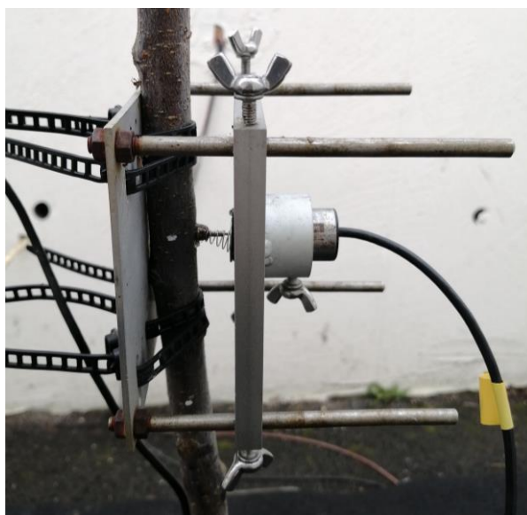
Figure 29: Microdendrometer mounted on the trunk of a studied tree in 2022.
