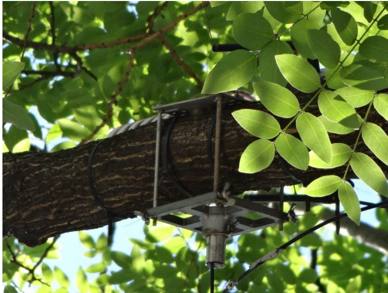
Figure 57: Picture of one microdendrometer mounted on a studied branch.
