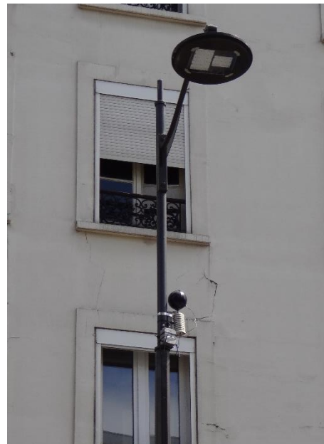
Figure 56: Pictures of the meteorological sensors mounted on two branches of one of the studied trees (left) and on one reference lamp post (right).
