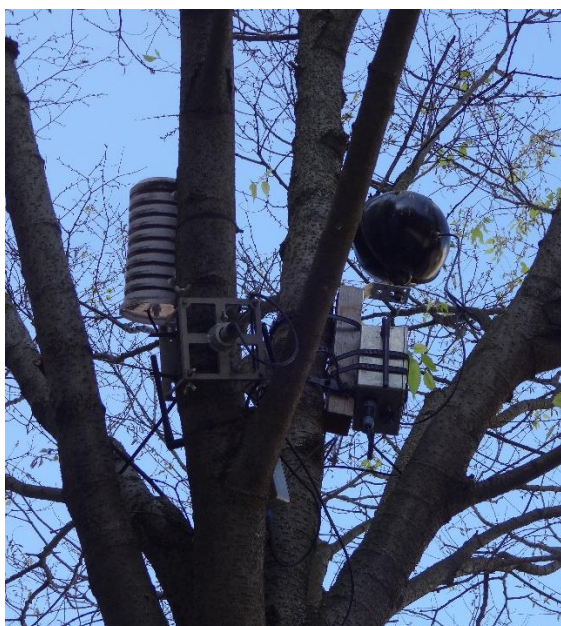
Figure 56: Pictures of the meteorological sensors mounted on two branches of one of the studied trees (left) and on one reference lamp post (right).
