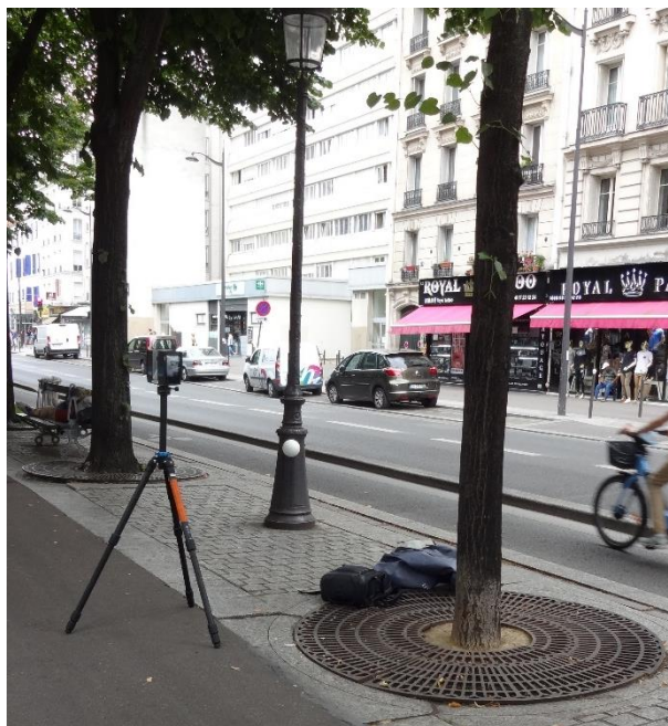
Figure 60: Picture of the FARO Focus 3D X130 mounted on a tripod scanning one of the studied trees.
