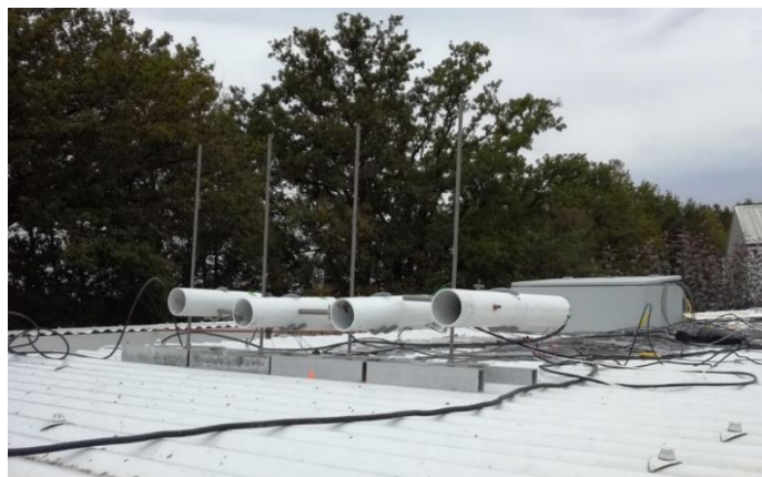
Figure 95: Picture of the air temperature and relative humidity sensors placed in mechanically ventilated white painted cylindrical shelters, initially mounted at 0.4 m a.g.l. on the central axis of the street in the NV, WW and WR zones, being compared on the roof of the eastern building of the canyon street. The additional sensor appearing on the picture was not studied in the frame of the present project.
