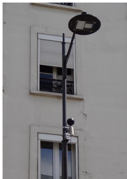
Figure 56: Pictures of the meteorological sensors mounted on two branches of one of the studied trees (left) and on one reference lamp post (right).
